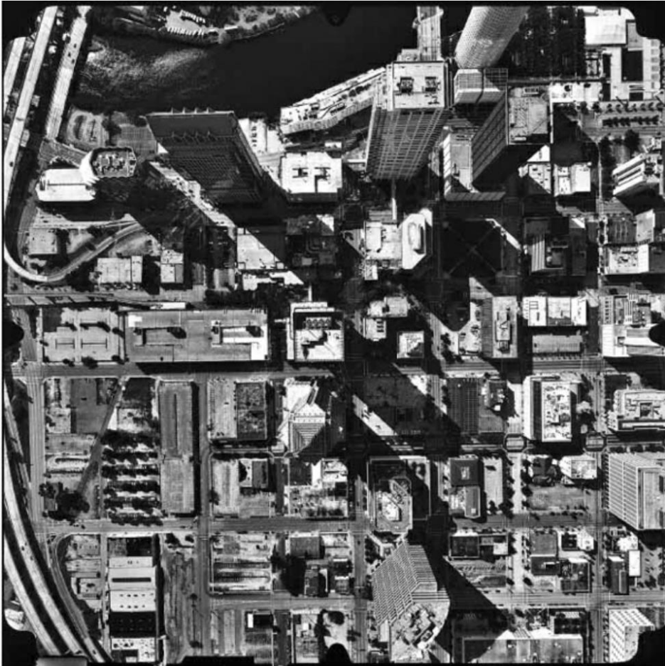
FIGURE 6-7 Vertical photograph of Tampa, Florida, illustrating relief displacements.
