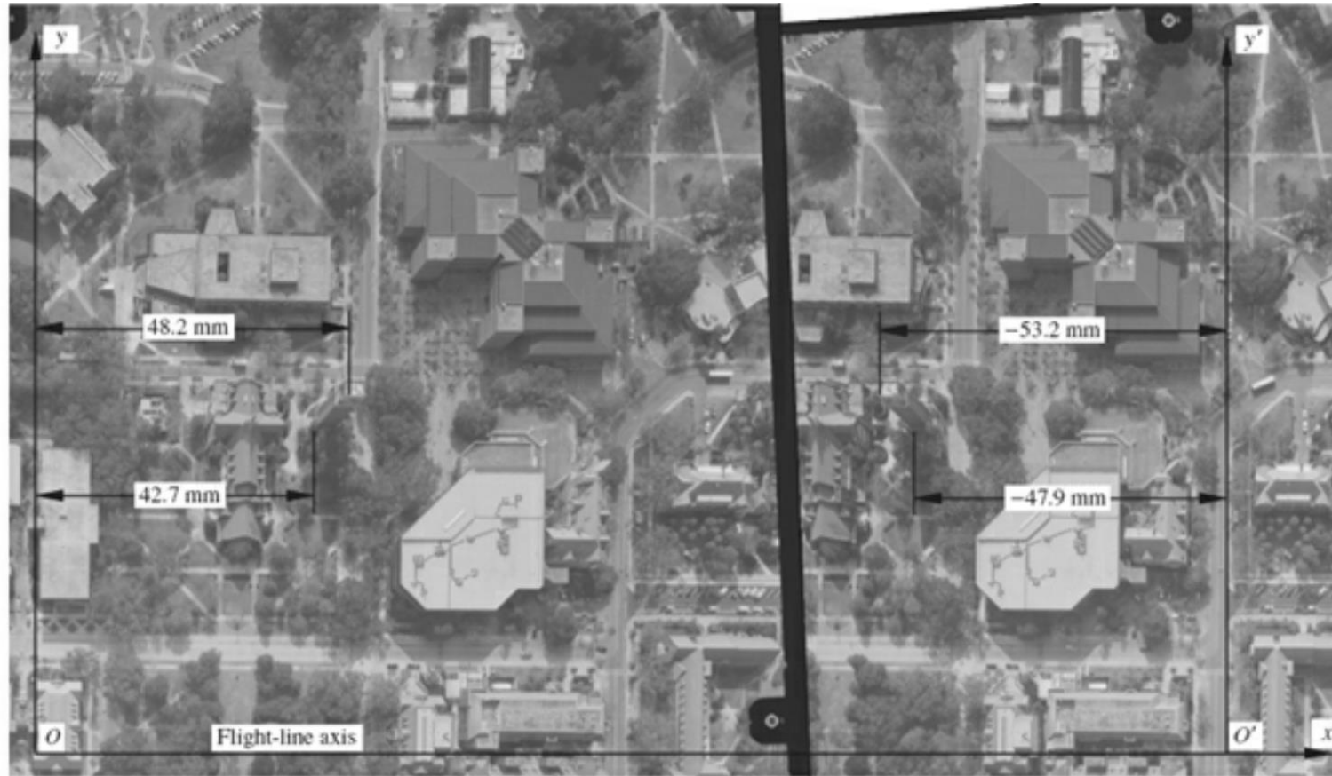
FIGURE 8-3 Overlapping vertical photographs taken over the University of Florida campus illustrating stereoscopic parallax.
