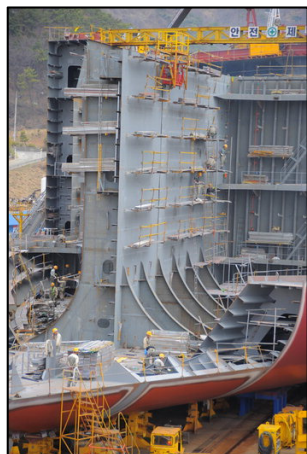
Example of hull structure of midship region
