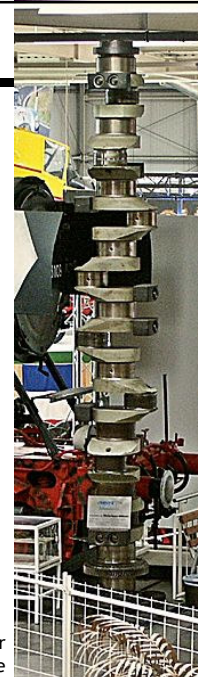
Crank shaft for 6-cylinder marine diesel engine
