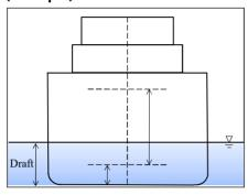
When winds of high velocity exist, beam winds and rolling are considered simultaneously.
