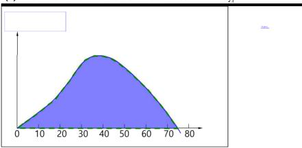
The total area between the statical stability curve (at zero degree to the angle of vanishing stability) and the horizontal axis represents from the upright position.
