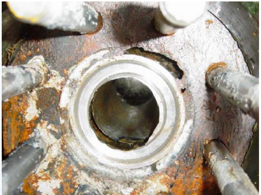
Tree failure (Sand erosion damage)
