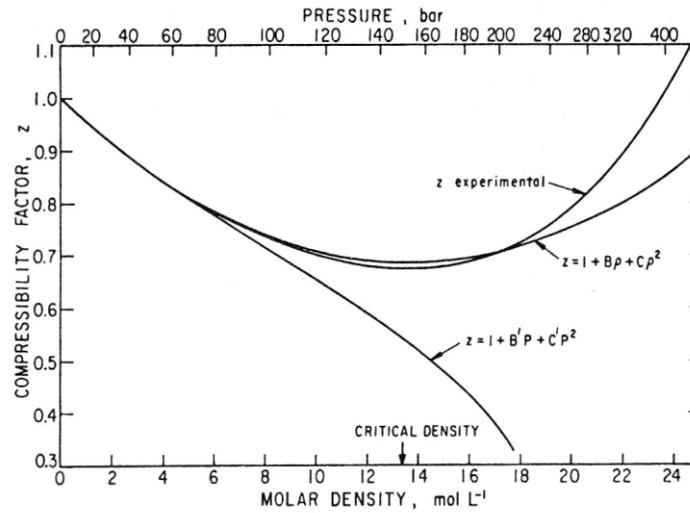
Figure 5-4 Compressibility factor for argon at  $-70^\circ\text{C}$ .
