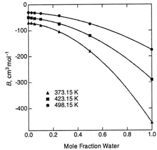
**Figure 5-6** Experimental second virial coefficients for the CO<sub>2</sub>/H<sub>2</sub>O system as a function of the mole fraction of water, for various temperatures (Patel *et al.*, 1987).
