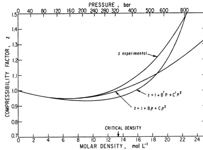
Figure 5-5 Compressibility factor for argon at  $25^\circ\text{C}$ .
