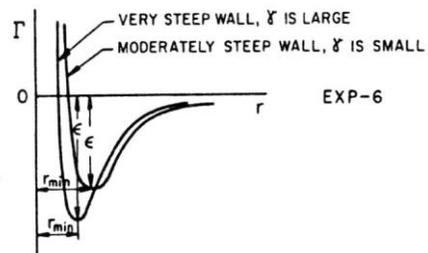
$\gamma$  determines the steepness of the repulsive wall.
