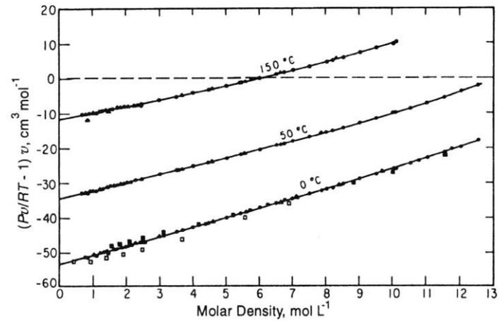
**Figure 5-2** Reduction of  $P$ - $V$ - $T$  data for methane to yield second and third virial coefficients (data from various sources).
