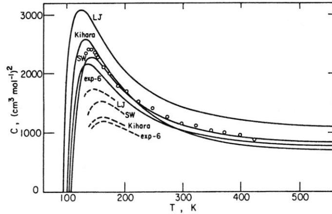
**Figure 5-19** Calculated and observed third virial coefficients for argon. Solid lines include Axilrod-Teller nonadditivity corrections. Dashed lines show a portion of calculated results assuming additivity. Circles represent experimental data of Michels (1958).
