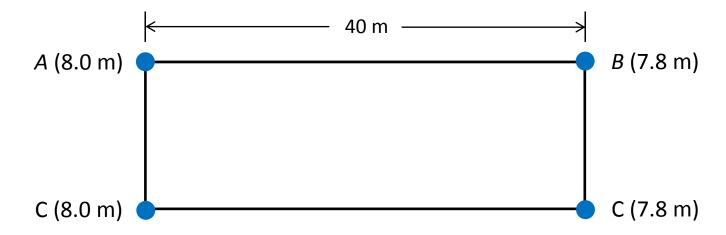
Determine the direction of the flow and the hydraulic gradient.
