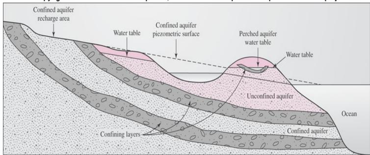
Confined aquifer: an aquifer bounded by impermeable layers both at the top and the bottom
