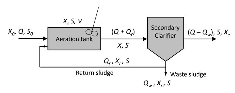
X,  $X_e$ ,  $X_r$ : MLVSS concentrations in aeration tank, effluent, and return sludge
