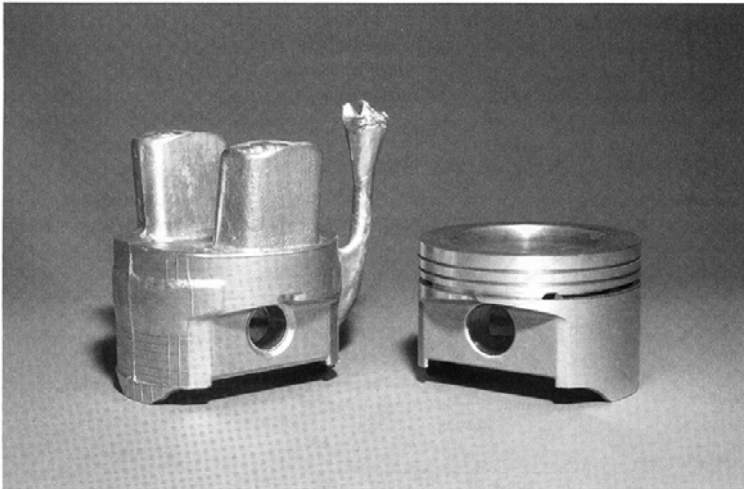
FIGURE 5.43 Aluminum piston for an internal combustion engine. (a) As cast; (b) after machining.
