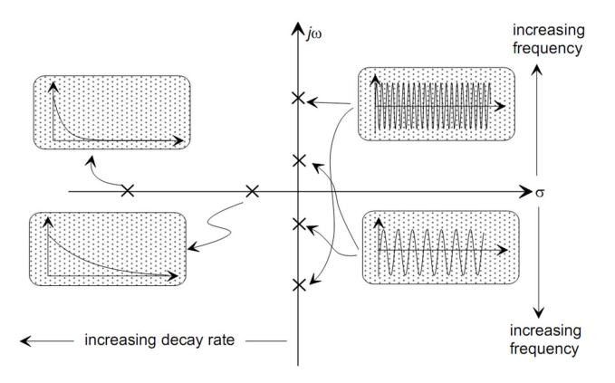
5) the oscillatory frequency and decay rate is determined by the distance of the poles from the origin.
