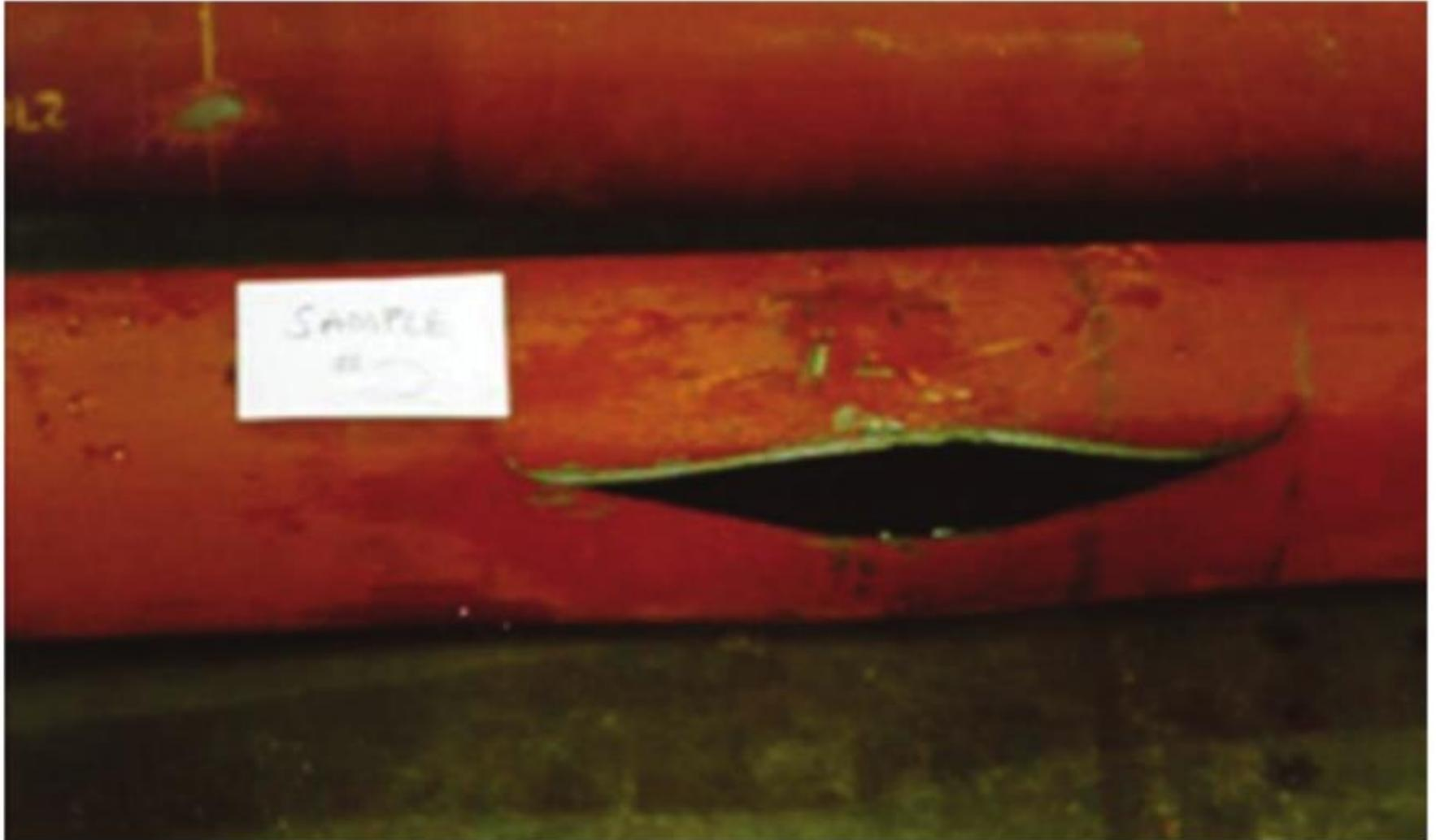
Figure A.1—Ductile Burst Sample
