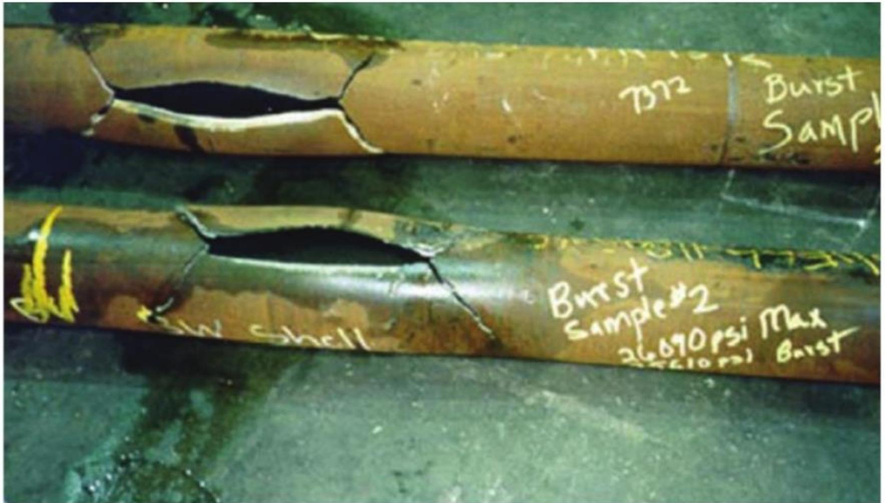
Figure A.2—Brittle Burst Sample
