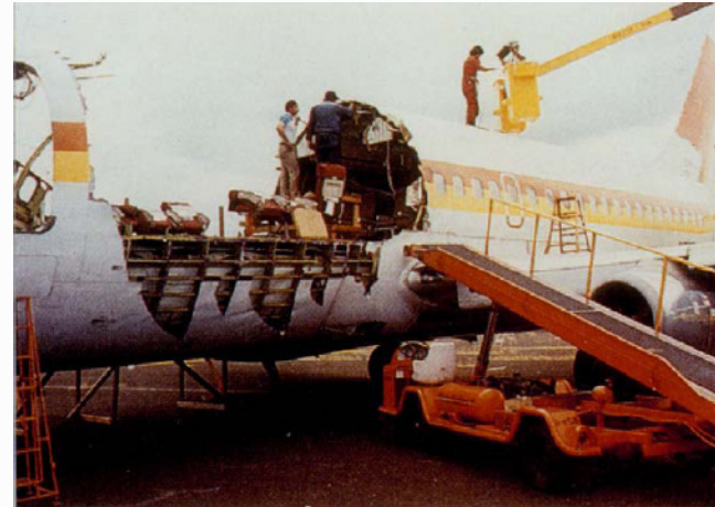
Fig.1.4 Aloha Airlines Flight 243, Boeing 737-200, April 28 1988, Honolulu, Hawaii (undetected cracks in fuselage skin, corrosion in the joint as a result of disbonding)
