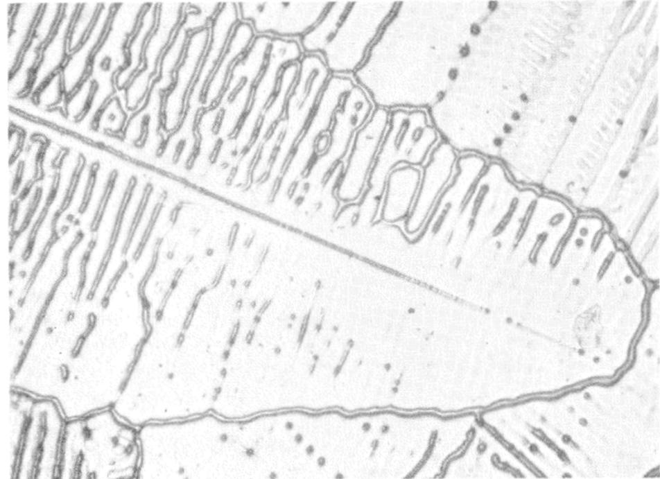
Fig. 5.45. Segregation in Al-Cu alloy
