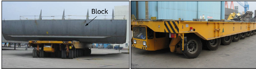
(a) Transporter with loading (b) Transporter without loading
