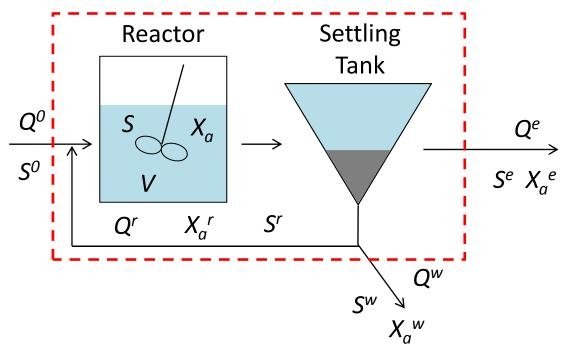
From flow mass balance:  $Q^0 = Q^e + Q^w$
