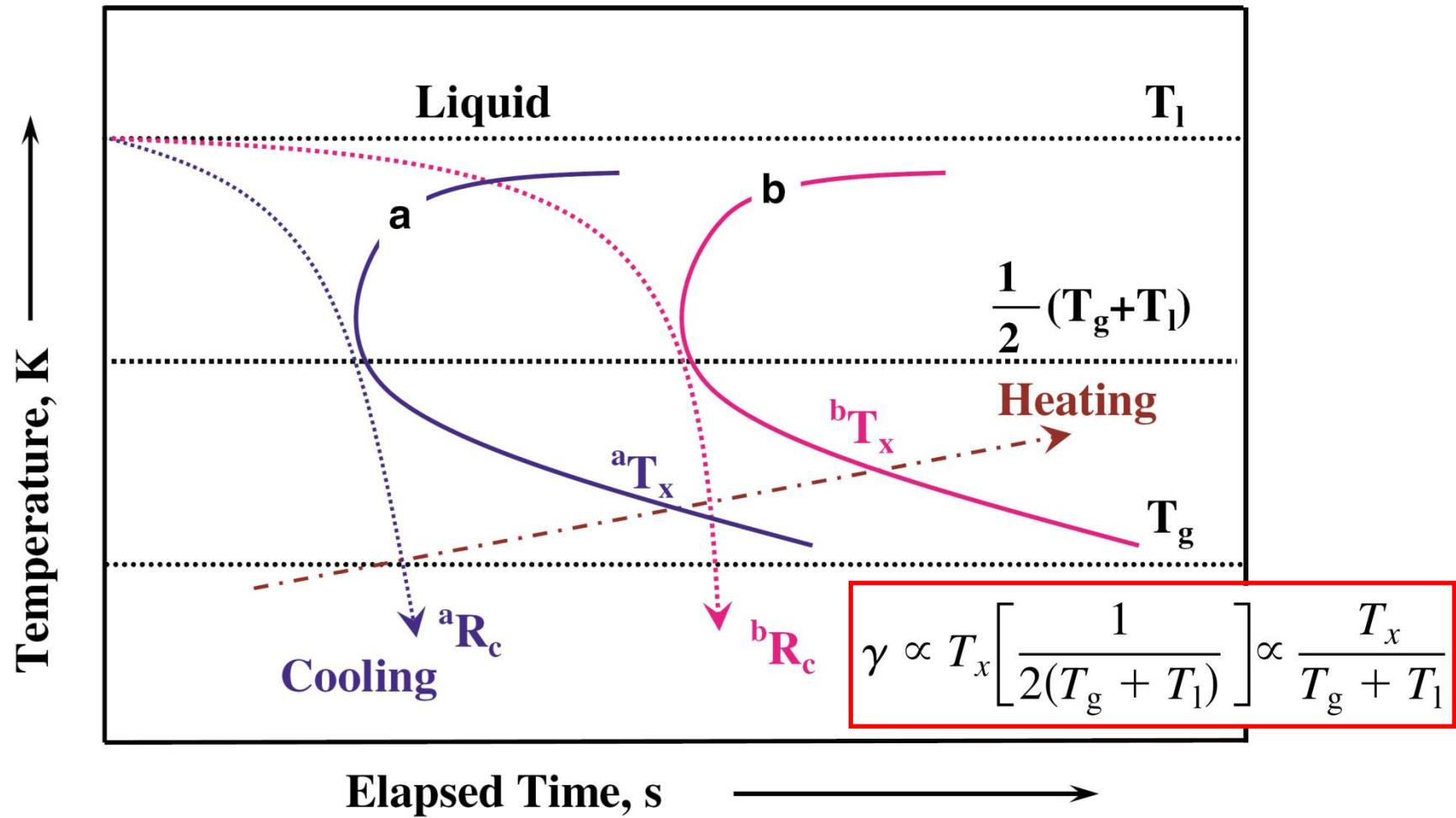
FIG. 2 (color online). Schematic TTT curves showing the effect of  $T_x$  measured upon continuous heating for different liquids with similar  $T_l$  and  $T_g$ ; liquid  $b$  with higher onset crystallization temperature  ${}^bT_x$  ( ${}^aT_x < {}^bT_x$ ) shows a lower critical cooling rate  ${}^bR_c$  ( ${}^bR_c < {}^aR_c$ ).
