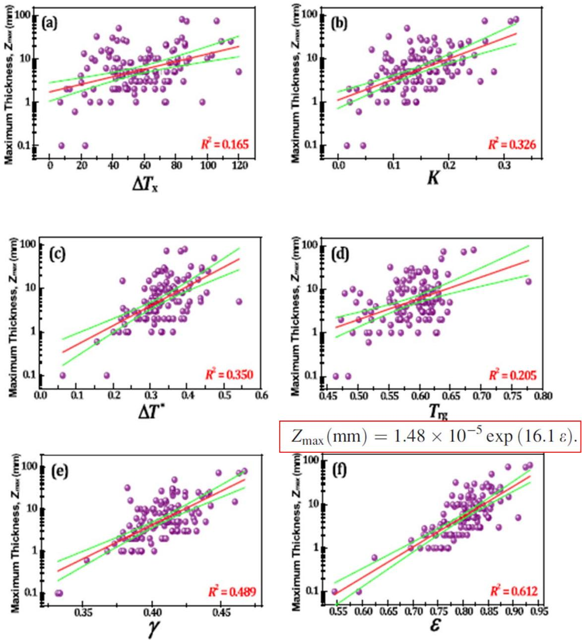
FIG. 5. A correlation between the parameters for GFA ( $\Delta T_x$ ,  $K$ ,  $T_{\text{rg}}$ ,  $\Delta T^*$ ,  $\gamma$ , and  $\epsilon$  parameters) and  $Z_{\max}$  for the various BMG-forming alloy systems reported previously.
