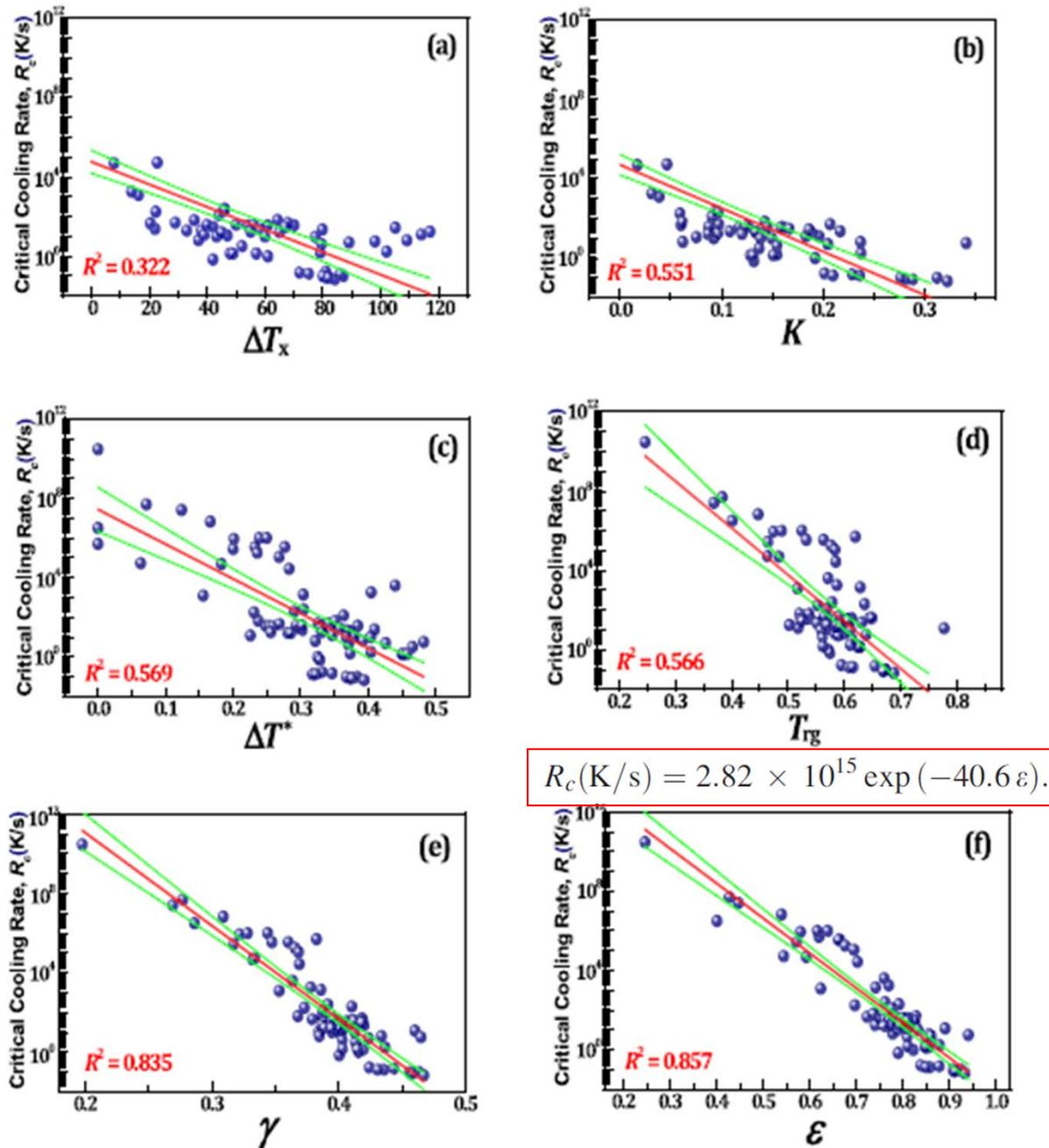
FIG. 4. A correlation between the parameters for GFA ( $\Delta T_x$ ,  $K$ ,  $T_{rg}$ ,  $\Delta T^*$ ,  $\gamma$ , and  $\varepsilon$  parameters) and  $R_c$  for the various glass-forming alloy systems reported previously.
