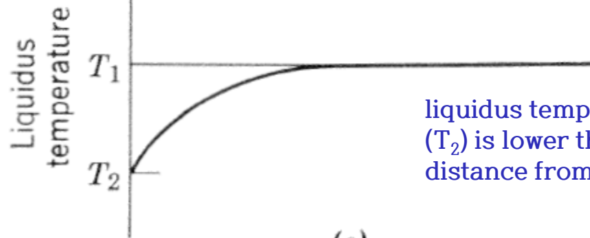
Fig. 5.26. Variation of concentration and liquidus temperature ahead of an interface. (a) Variation of concentration, (b) relationship between concentration and liquidus temperature, (c) variation of liquidus temperature.
