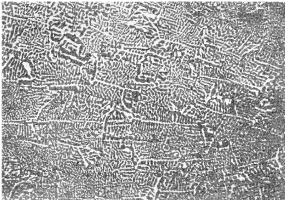
Fig. 6.25. “Chinese script” structure in Bi-Sn eutectic alloy
