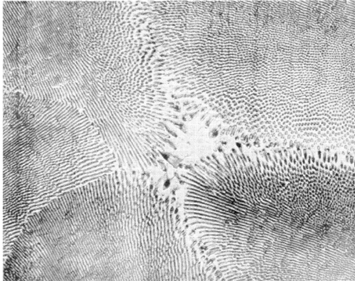
Fig. 6.24. "Mixed lamellar and rod structure" (Pb-Cd eutectic alloy with 0.1% Sn)
