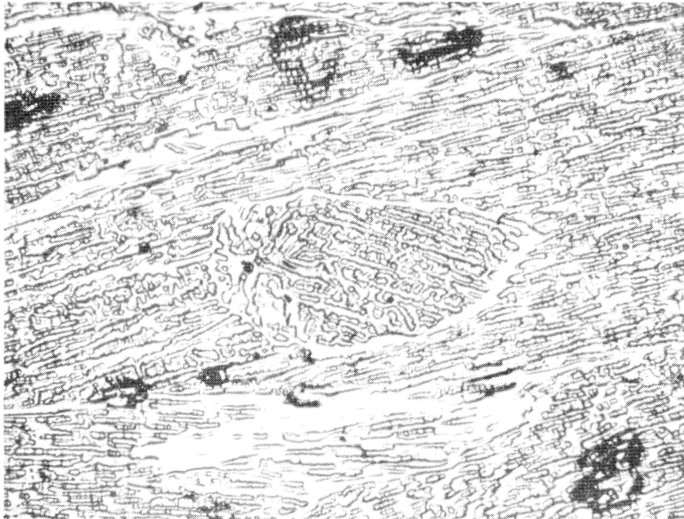
Fig. 8.12. Equiaxed crystals in columnar zone.
