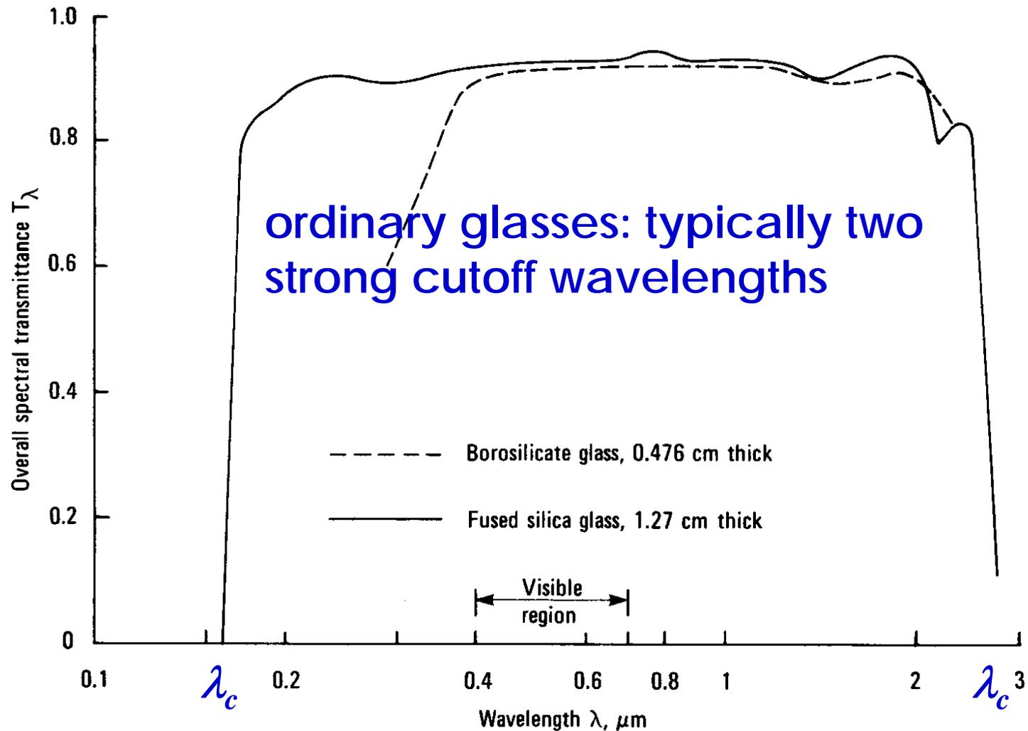
Normal overall spectral transmittance of glass plate (includes surface reflection) at 298 K
