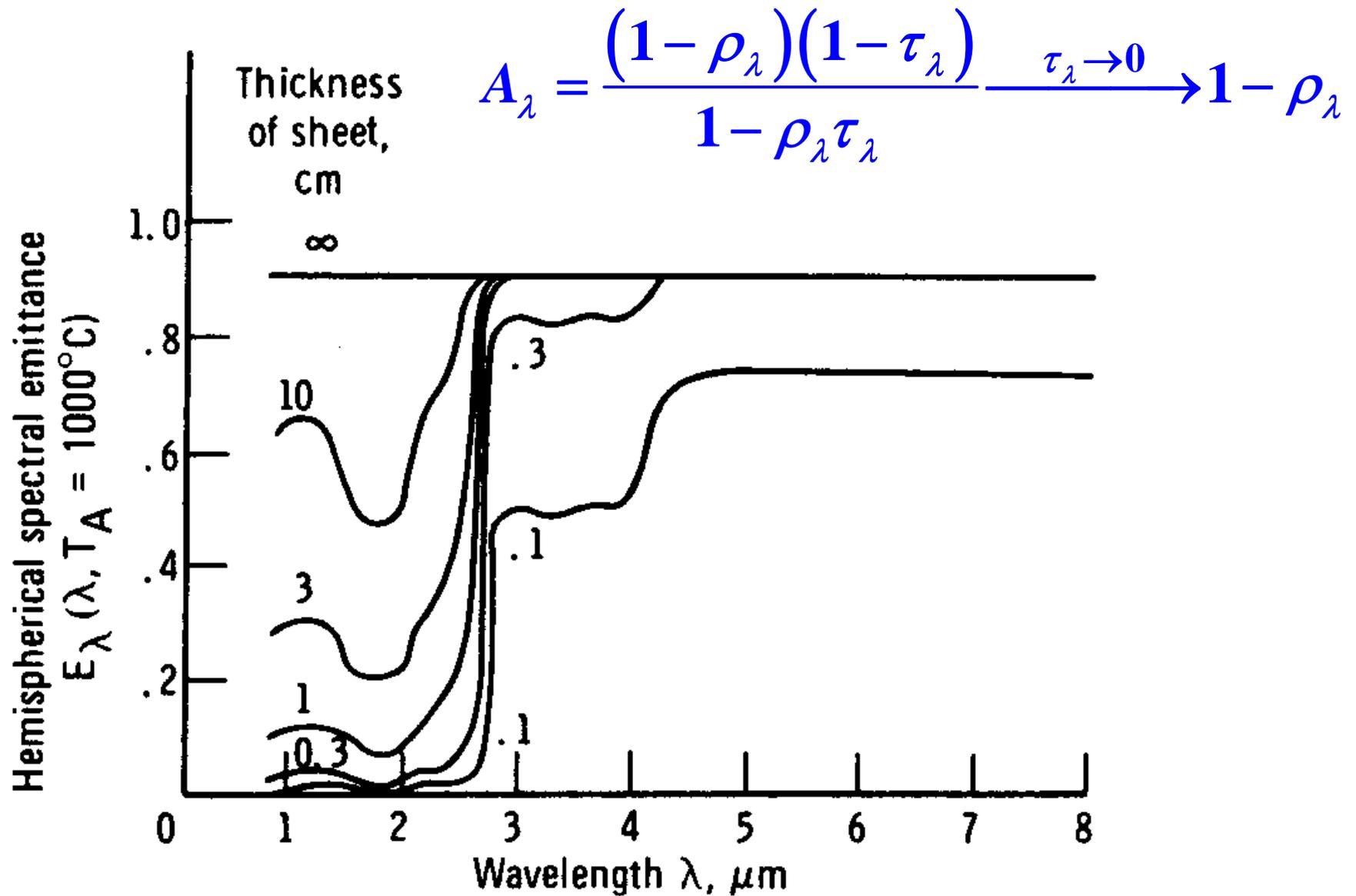
Emittance of sheets of window glass at  $1000^\circ\text{C}$
