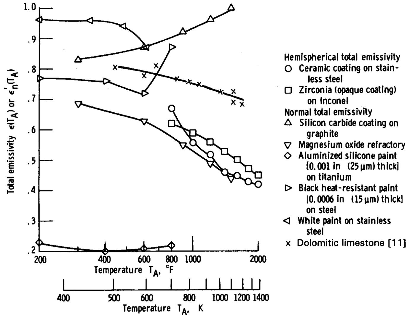
Effect of surface temperature on emissivity of dielectrics
