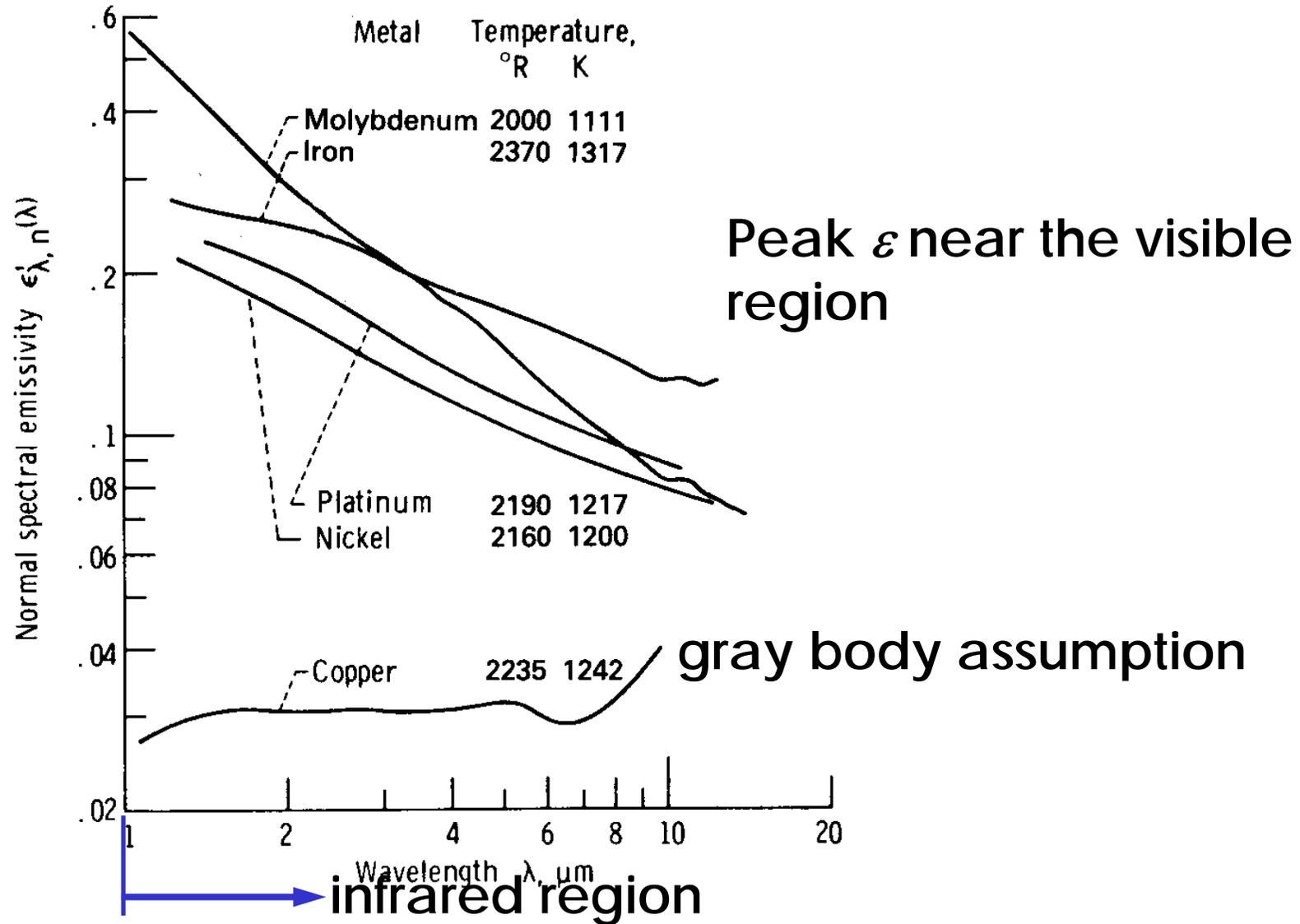
Variation with wavelength of normal spectral emissivity for polished metals
