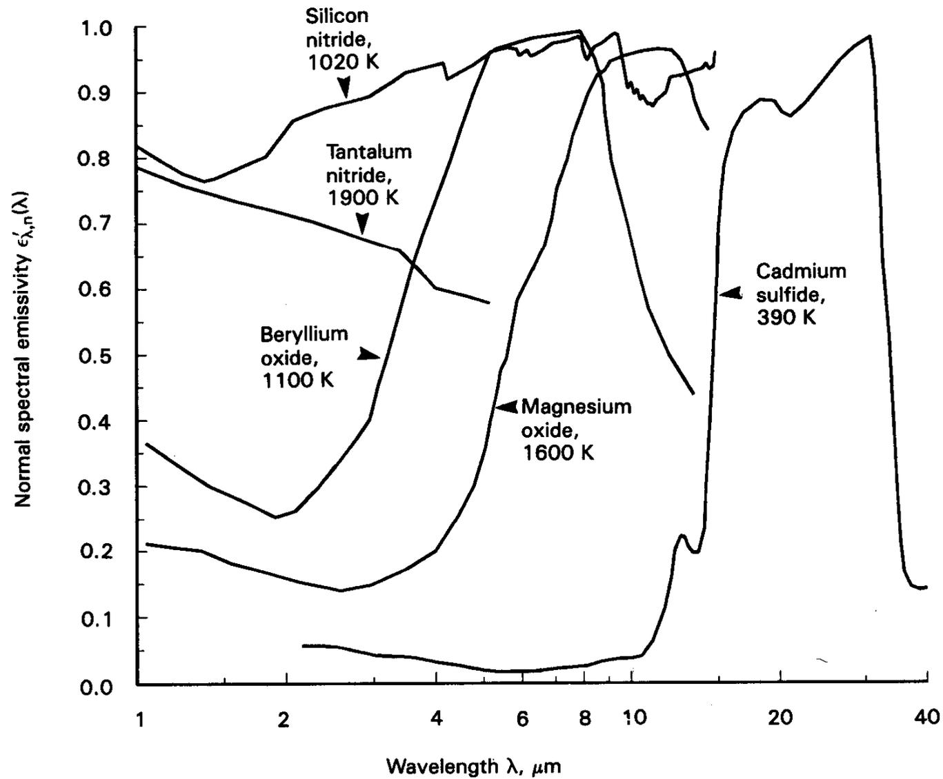
Normal spectral emissivity of some nonmetal samples.
