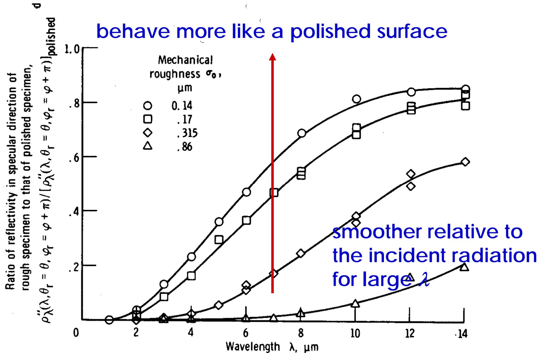
Effects of roughness on bidirectional reflectivity in specular direction for ground nickel specimens. Mechanical roughness for polished specimen,  $0.015 \mu\text{m}$
