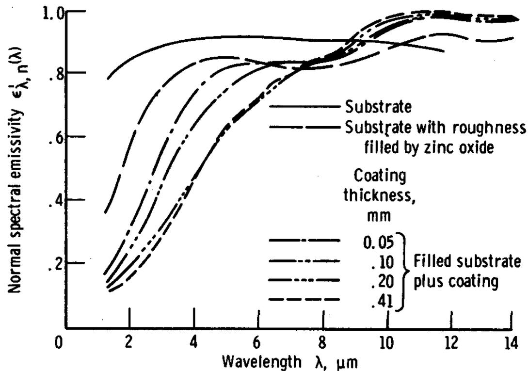
Emissivity of zinc oxide coatings on oxidized stainless steel substrate. Surface temperature,  $880 \pm 8 \text{ K}$
