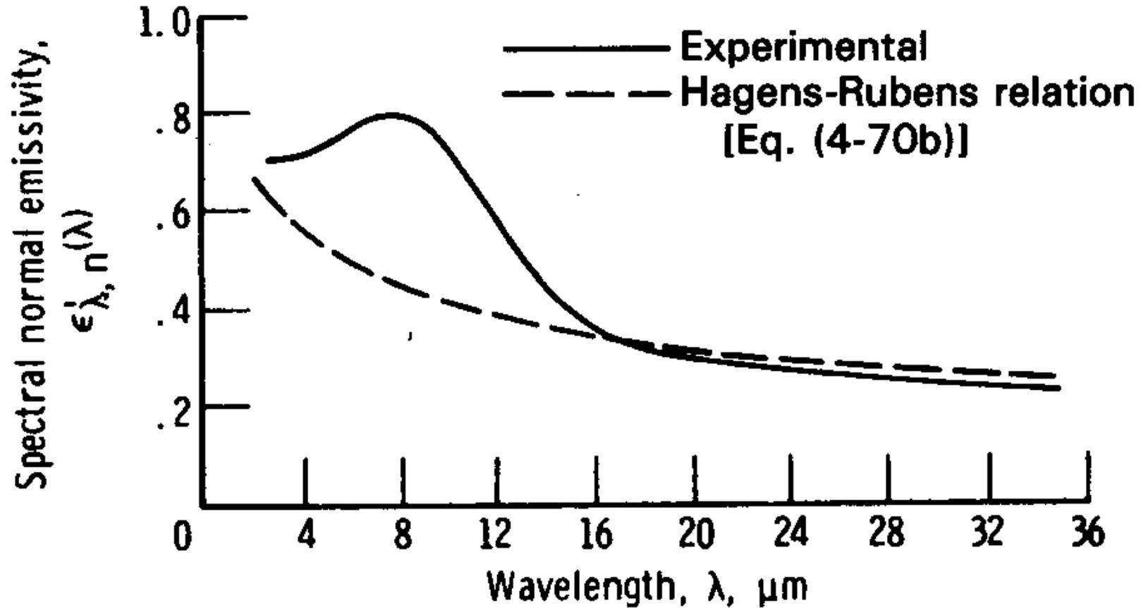
Normal spectral emissivity of a highly doped silicon semiconductor at room temperature
