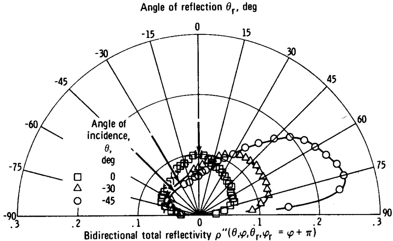
Bidirectional total reflectivity of typewriter paper in plane of incidence. Source temperature, 1178 K
