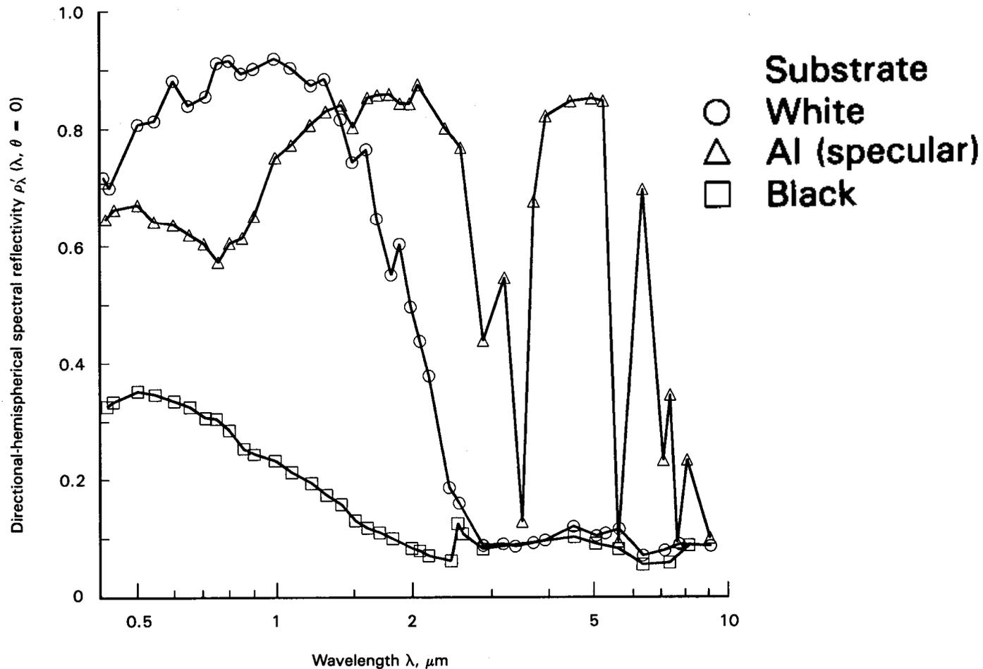
Effect of substrate reflection characteristics on the hemispherical characteristics of a  $\text{TiO}_2$  paint film for normal incidence: Film thickness,  $14.4 \mu\text{m}$ ; volume concentration of pigment **0.017**,
