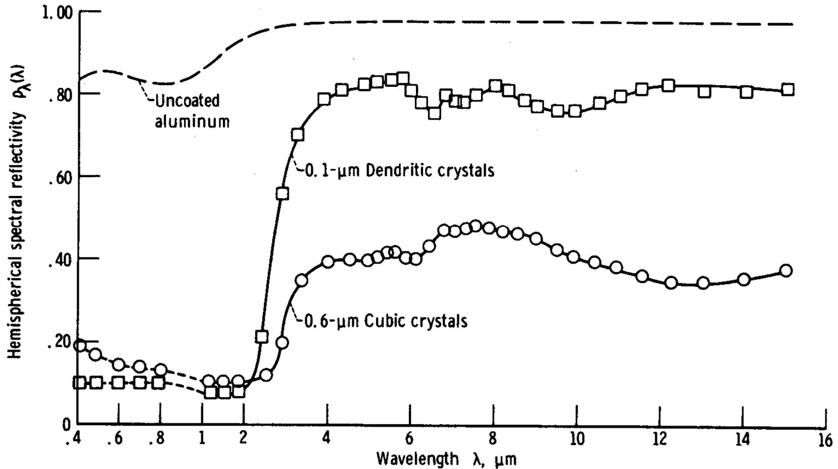
Hemispherical spectral reflectivity for normal incident beam on aluminum coated with lead sulfide. Coating mass per unit surface area,  $0.68 \text{ mg/cm}^2$
