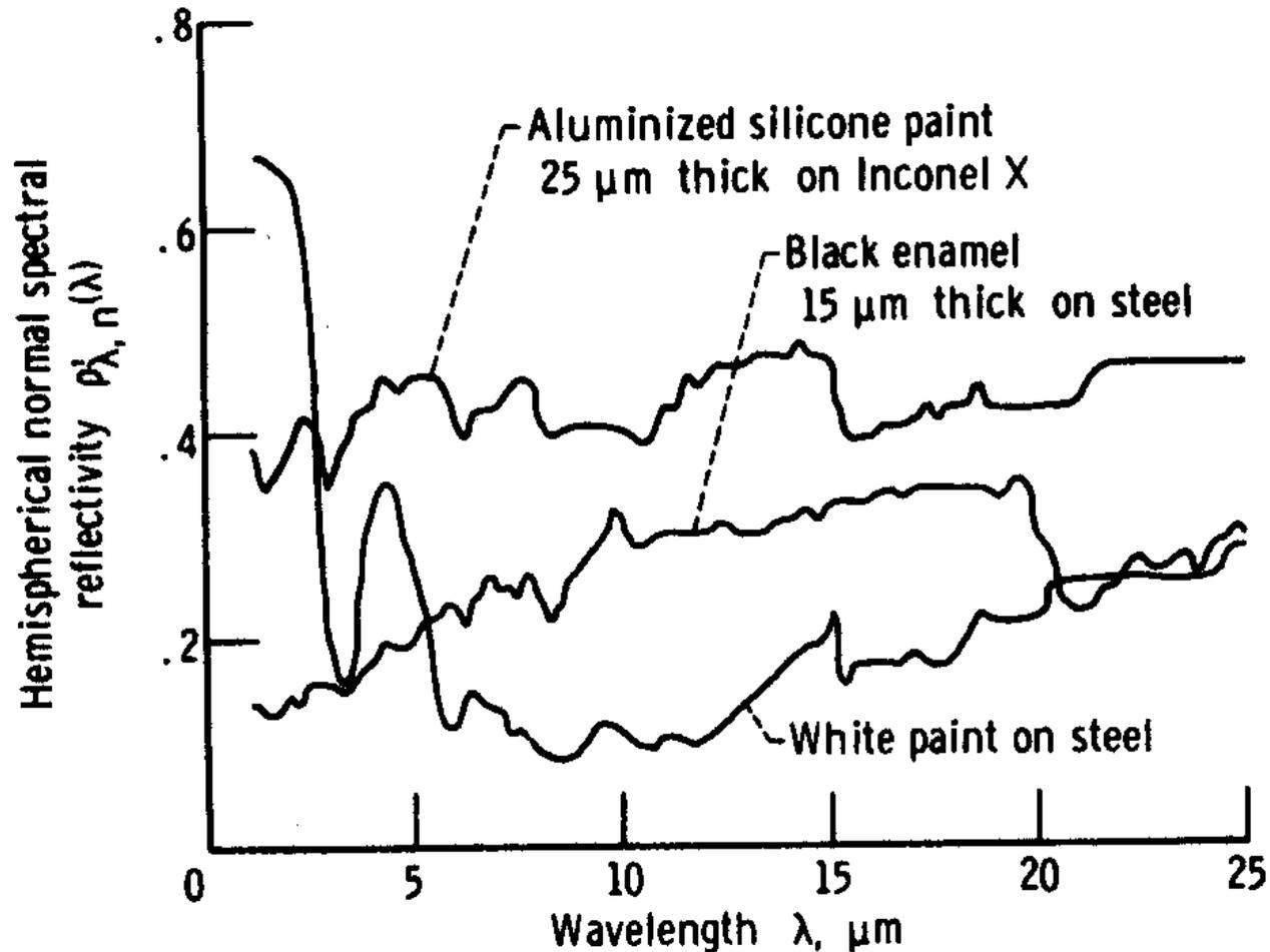
Spectral reflectivity of paint coatings. Specimens at room temperature
