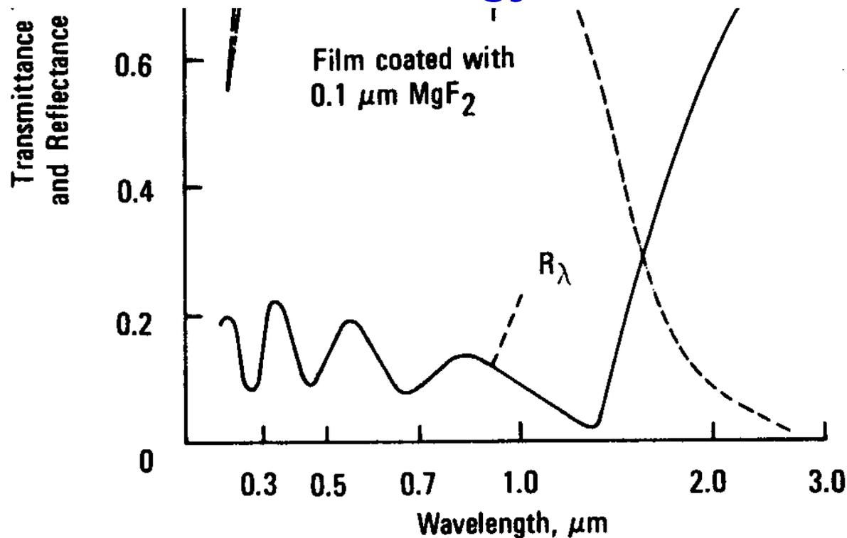
Transmittance and reflectance of 0.35- $\mu\text{m}$ -thick film of Sn-doped  $\text{In}_2\text{O}_3$  film on Corning 7059 glass. Also shown is the effect on  $T_\lambda$  of an antireflection coating of  $\text{MgF}_2$
