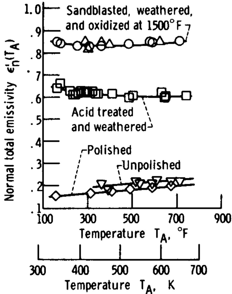
Effect of surface condition and oxidation on normal total emissivity of stainless steel type 18-8
