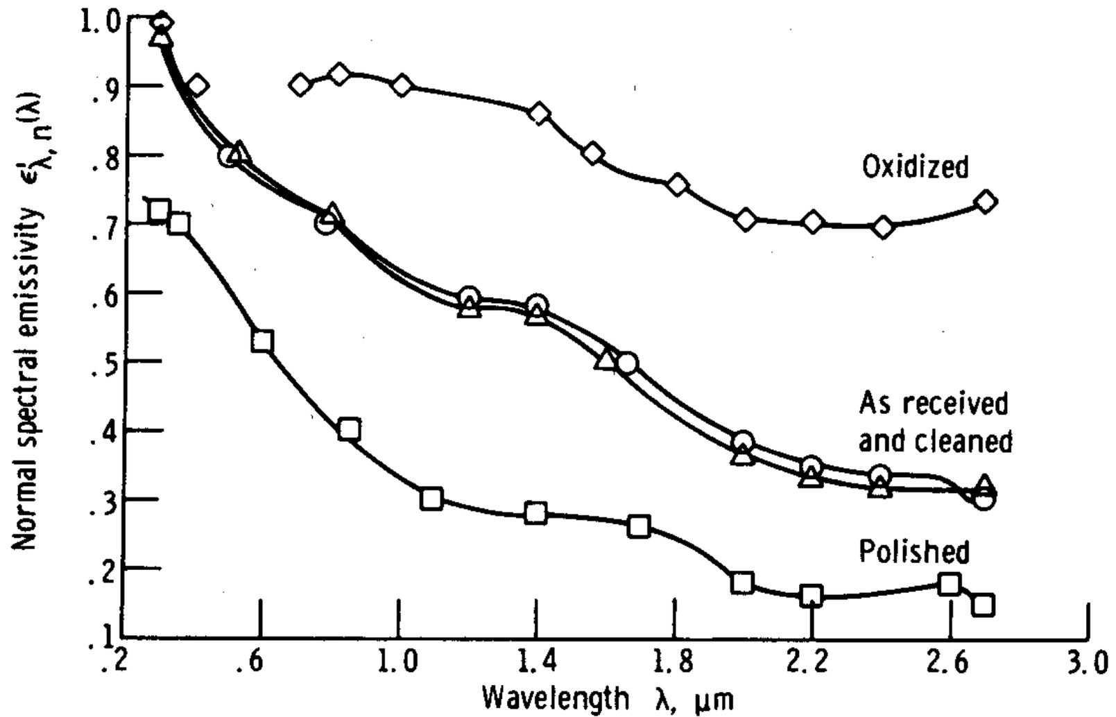
Effect of oxidation on normal spectral emissivity of Inconel X
