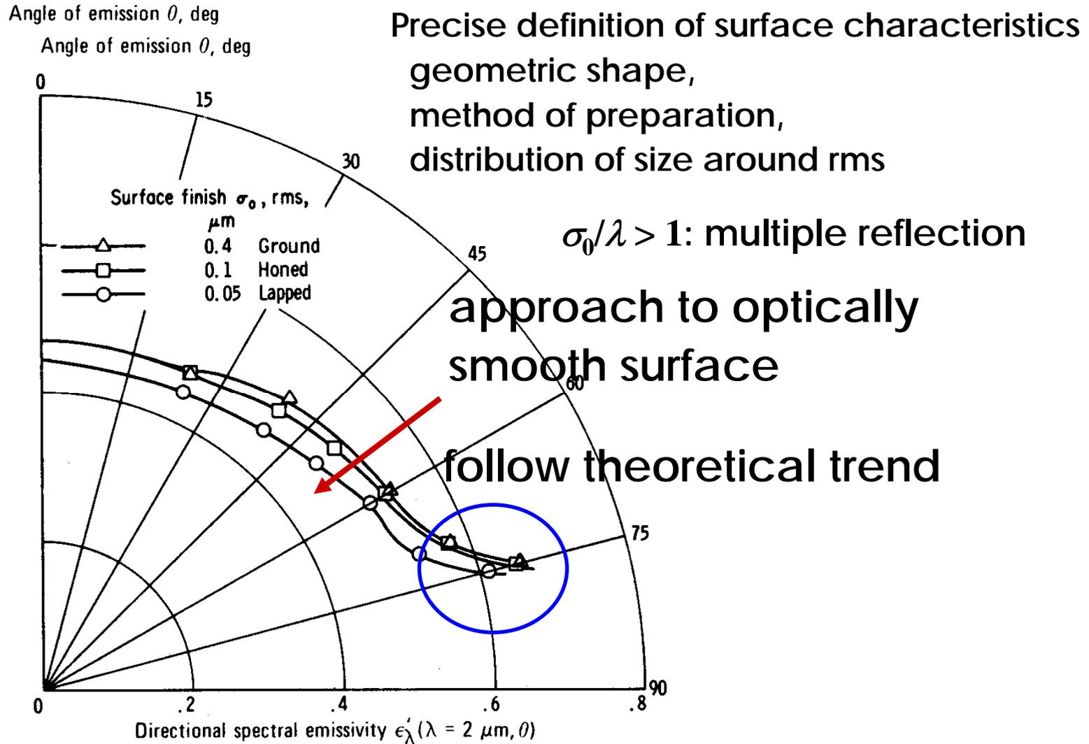
Roughness effects for small optical roughness,  $\sigma_0/\lambda < 1$ ; effect of surface finish on directional spectral emissivity of pure titanium. Wavelength,  $2 \mu\text{m}$
