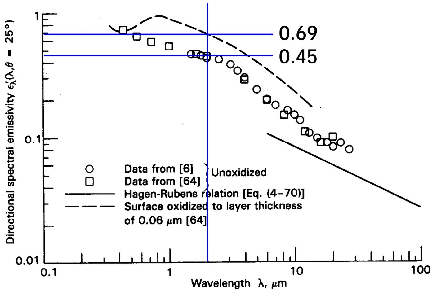
Effect of oxide layer on directional spectral emissivity of titanium. Emission angle,  $\theta = 25^{\circ}$ ; surface lapped to  $0.05 \mu\text{m}$  rms; temperature, 294 K.
