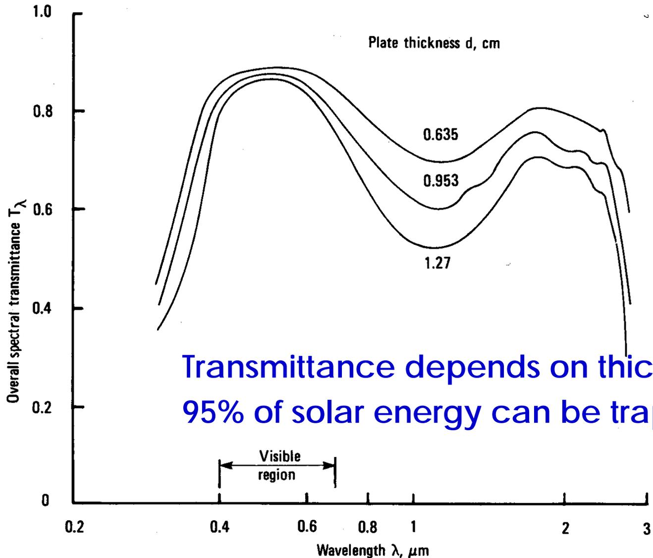
Transmittance depends on thickness.
