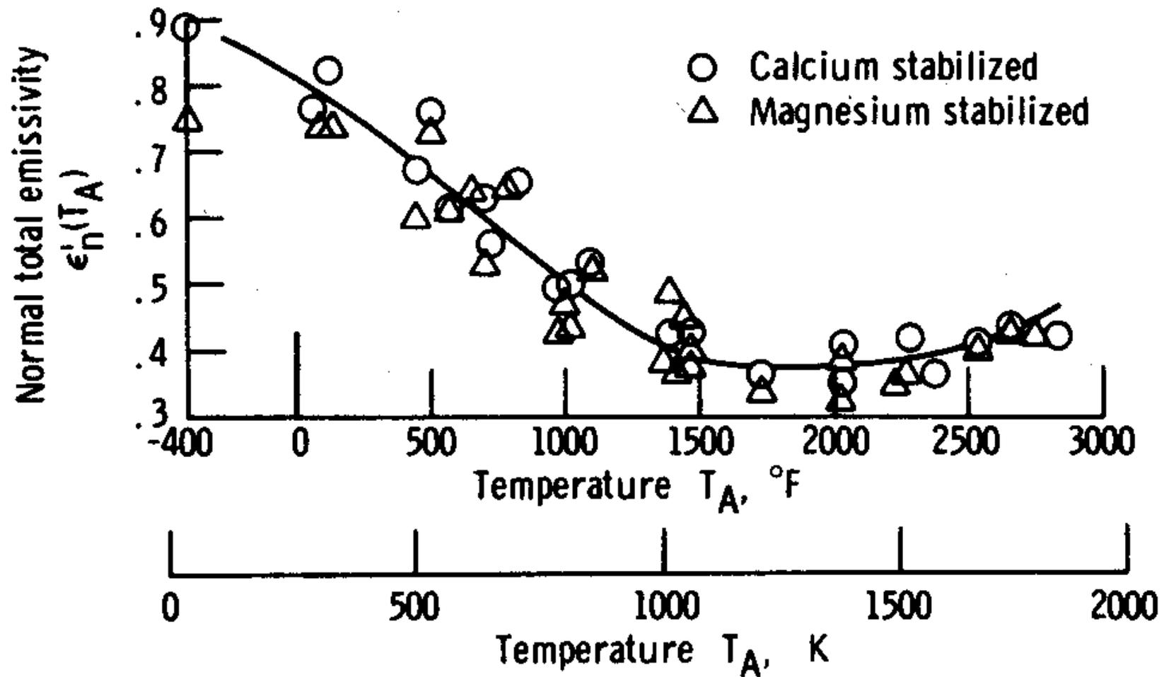
Effect of surface temperature on normal total emissivity of zirconium oxide
