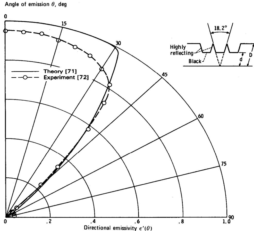
Directional emissivity of grooved surface with highly reflecting specular side walls and highly absorbing base;  $d/D = 0.649$ . Results in plane perpendicular to groove direction; data at  $8 \mu\text{m}$
