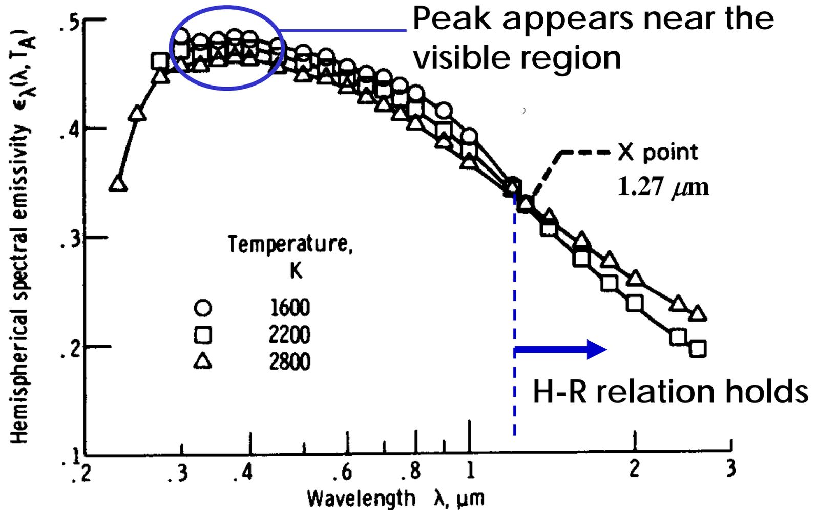
Effect of wavelength and surface temperature on hemispherical spectral emissivity of tungsten
