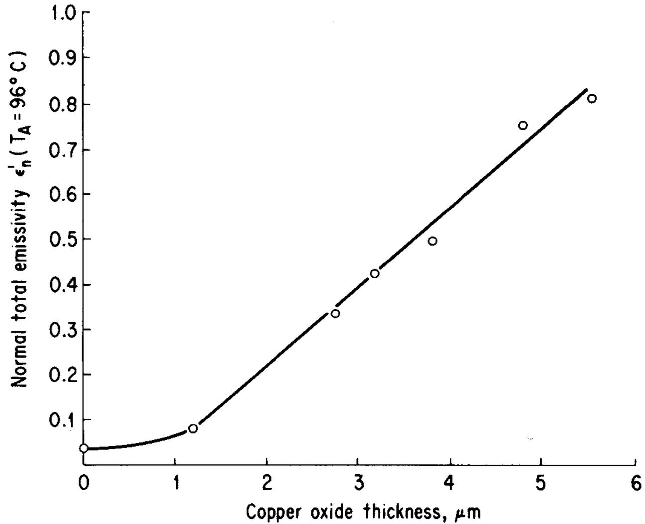
**Effect of oxide thickness on normal total emissivity of copper at 369 K**
