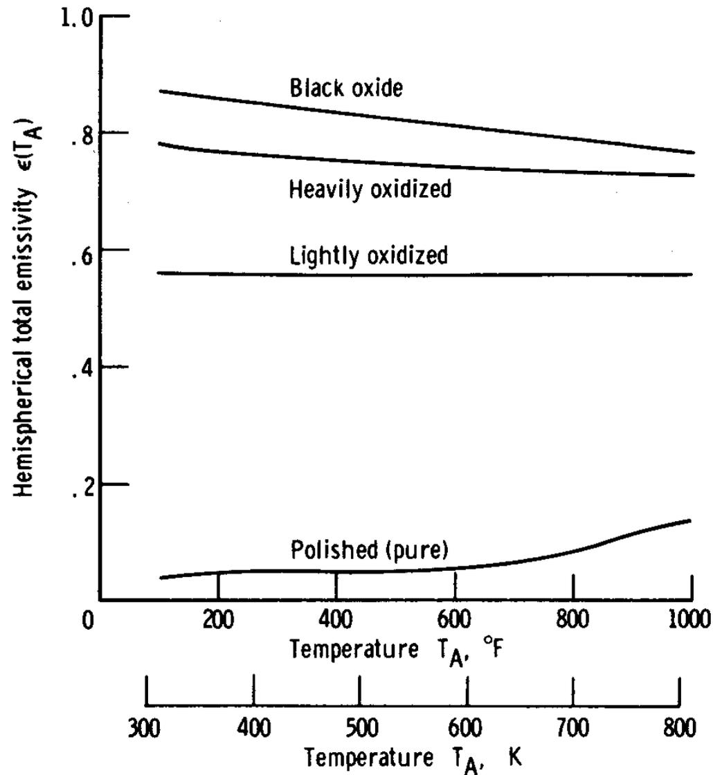
Effect of oxide coating on hemispherical total emissivity of copper
