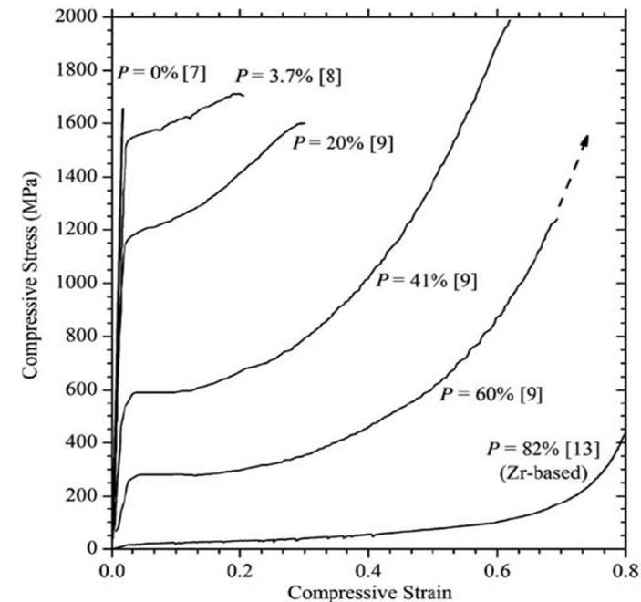
Figure 3. Compressive engineering stress–strain curves for several porous amorphous metals at intervals of approximately 20% porosity  $P$ . All but the highest-porosity material (which was processed from  $Zr_{57}Nb_5Cu_{15.4}Ni_{12.6}Al_{10}$ ) were processed from  $Pd_{42.5}Cu_{30}Ni_{7.5}P_{20}$ .
