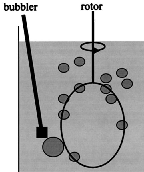
Schematic drawing of the eggbeater constructed for the mechanical air-entrapment method. The setup comprises a molybdenum brush of 3 cm diameter spinning at speeds of up to 2500 rpm.
