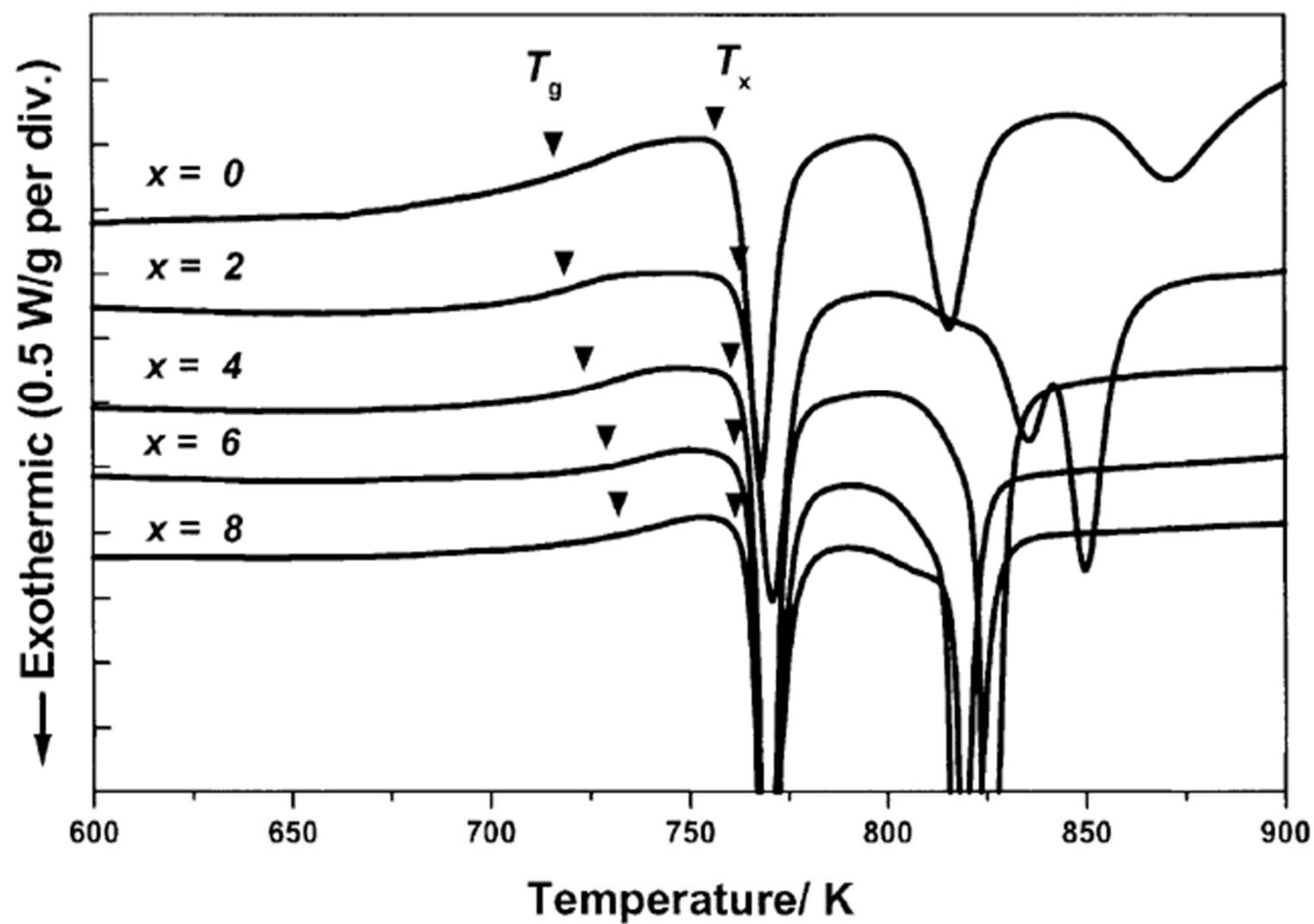
Fig. 1. DSC traces of rapidly solidified  $\text{Cu}_{47}\text{Ti}_{33}\text{Zr}_{11}\text{Ni}_{8-x}\text{Sn}_x\text{Si}_1$  ( $x = 0, 2, 4, 6, 8$ ) alloy ribbons obtained during heating with a heating rate 0.667 K/s.
