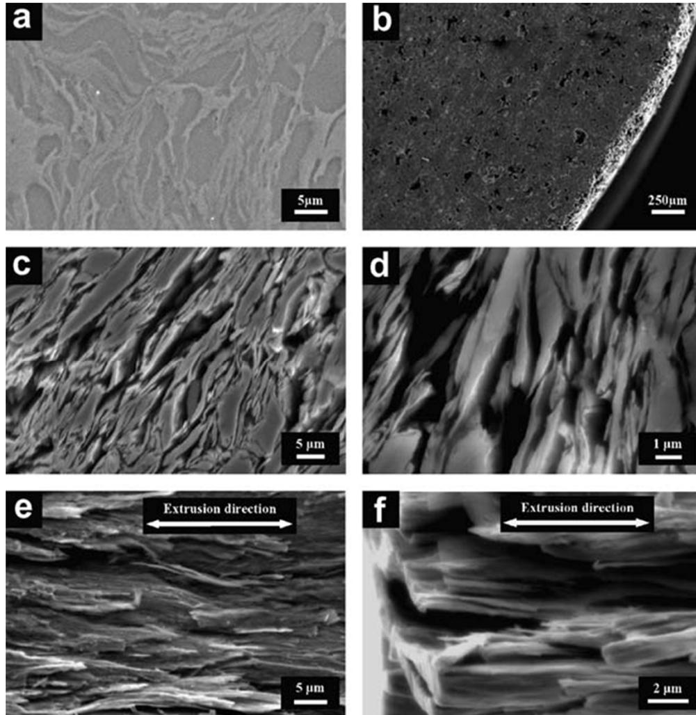
SEM images of porous  $\text{Cu}_{47}\text{Ti}_{33}\text{Zr}_{11}\text{Ni}_8\text{Si}_1$  MG. Pores are uniformly distributed throughout the sample.
