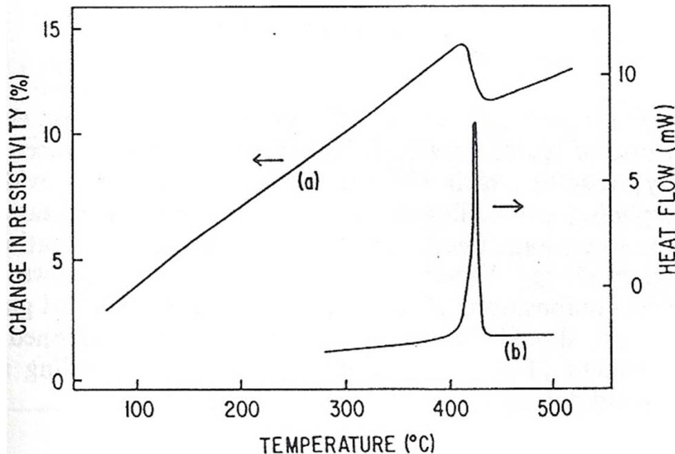
Figure 10.3 (a), Resistivity curve obtained by heating the glass  $\text{Fe}_{40}\text{Ni}_{40}\text{B}_{20}$  at 5 K/min from room temperature (courtesy of J. Rout). (b), DSC trace obtained under the same conditions
