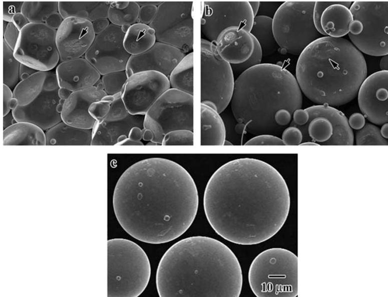
SEM micrographs of the transverse (mechanically crushed) cross section of the sintered porous  $Zr_{55}Cu_{30}Al_{10}Ni_5$  bulk glassy alloys with porosities of 4.7% (a), 33.5% (b), and the original powder (c).
