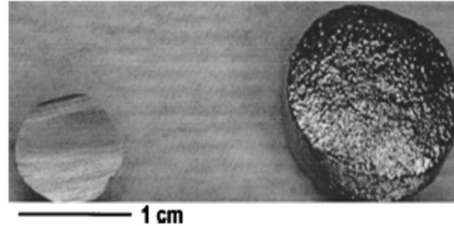
FIG. 11. Size comparison of  $\text{Pd}_{43}\text{Ni}_{10}\text{Cu}_{27}\text{P}_{20}$  prefoam (left) and expanded foam (right) by rf-coil. The bubble volume fraction of the prefoam is 10%, while that of the final foam is 75%.
