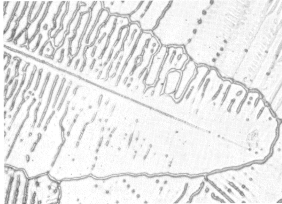
Fig. 5.45. Segregation in Al-Cu alloy
