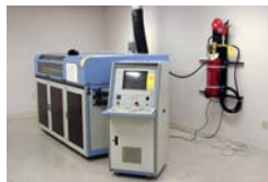
Helixsis 2030E LOM machine Part envelope size 32"x22"x20"
