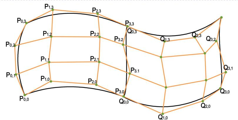
When two Bezier surfaces are connected, control points before and after connection should form straight lines to guarantee G1 continuity
