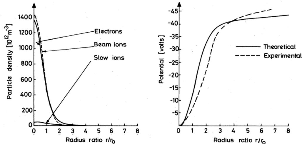
FIG. 4. Shape of the potential well and particle profiles at low pressure; beam energy 20-keV  $\text{He}^+$ , pressure  $1.25 \times 10^{-4}$  Torr, current 17.6 mA, radius 5 mm.
