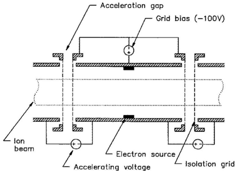
Bias grids prevent streaming of electrons into the acceleration gaps
