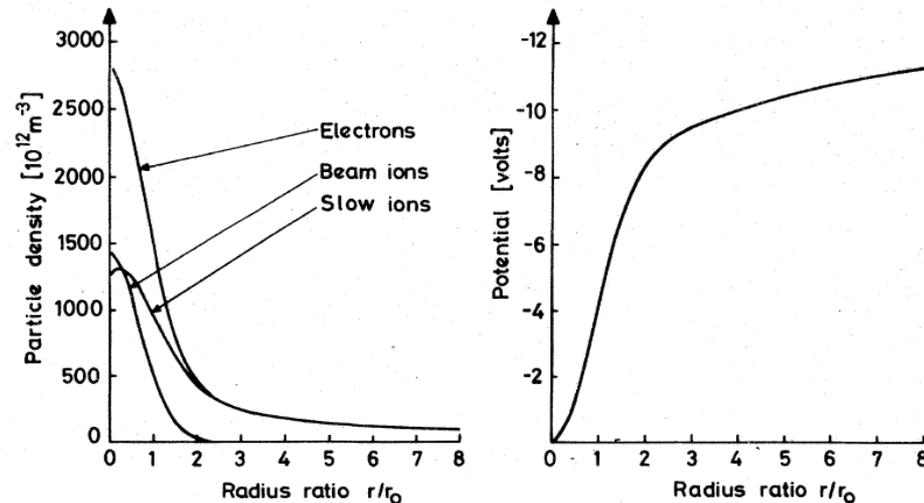
FIG. 5. Shape of the potential well and particle profiles at high pressure; beam energy 20-keV  $\text{He}^+$ , pressure  $2 \times 10^{-3}$  Torr, current 17.6 mA, radius 5 mm.
