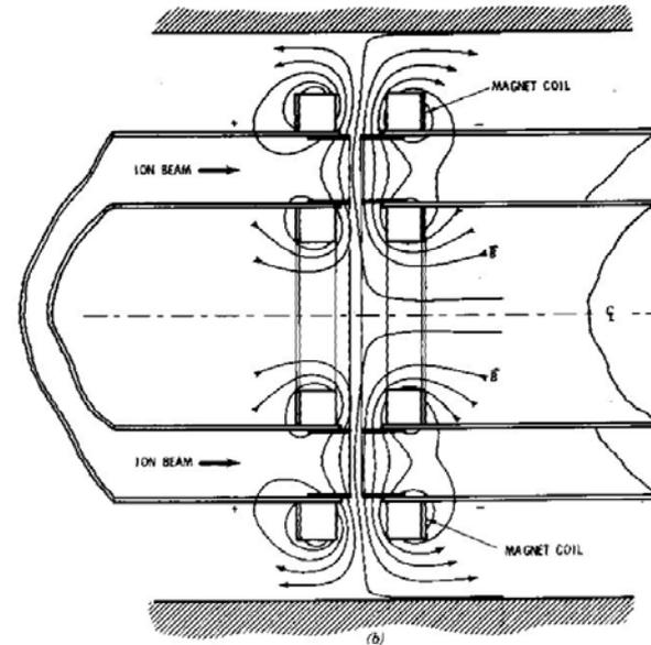
Radial magnetic field inhibits electron streaming
