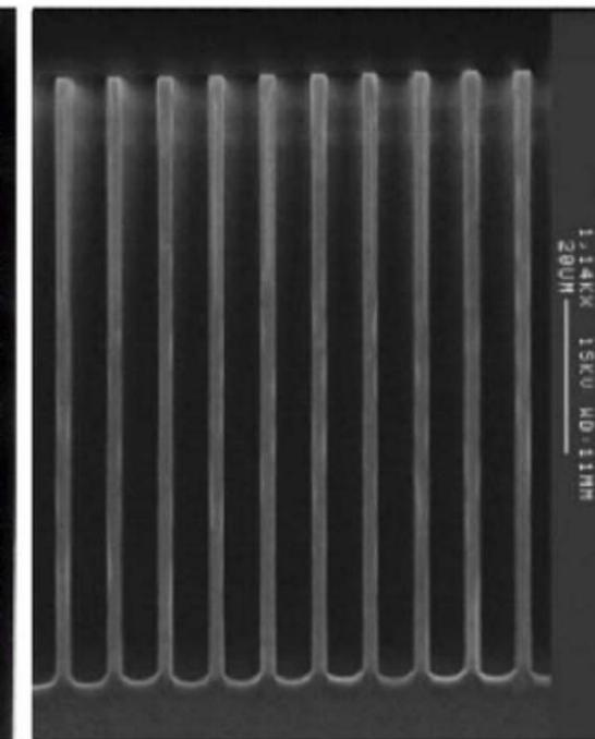
80  $\mu\text{m}$ -depth, 4.5  $\mu\text{m}$  space width, 2  $\mu\text{m}$  line width
