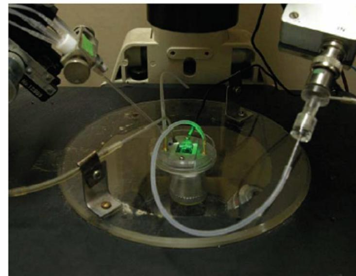
Setup with Patch clamping system
