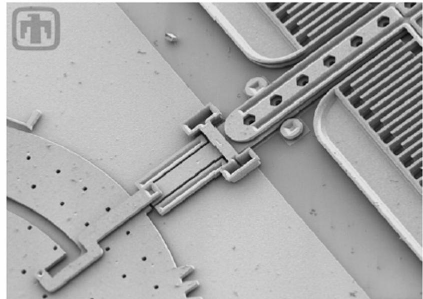
Micromechanical lock pin actuator
