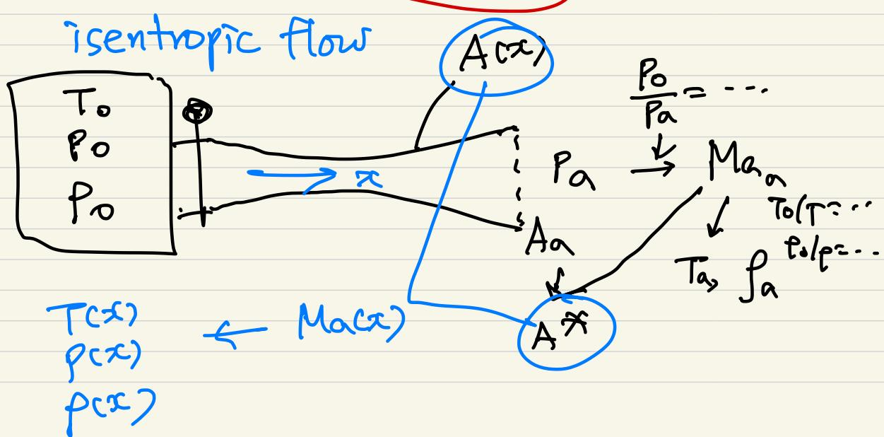
\* choking : for given stagnation conditions, the maximum possible mass flow passes through a duct when its throat is at the sonic condition. Then the duct is  $dA=0$  said to be choked and carry no additional mass flow.
