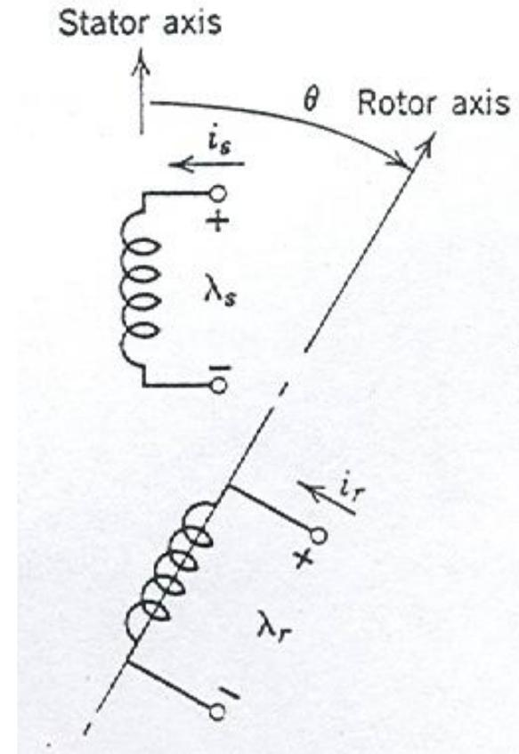
**Schematic representation of the inductors constituting the rotor and stator winding.**
