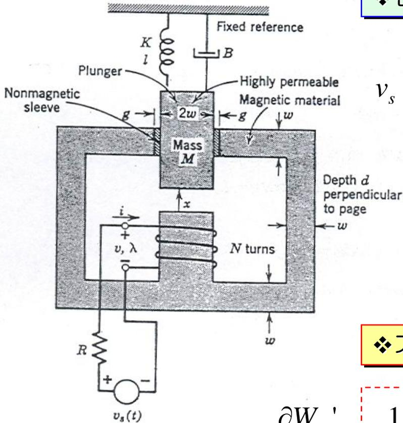
$$v_s = Ri + \frac{d\lambda}{dt} = Ri + \frac{\partial \lambda}{\partial i} \frac{\partial i}{\partial t} + \frac{\partial \lambda}{\partial x} \frac{\partial x}{\partial t}$$
