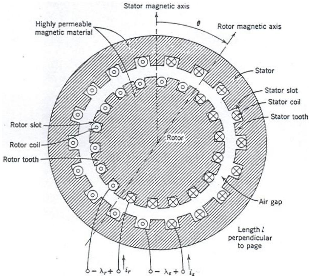
**Geometry of smooth-air-gap machine showing distributed windings on stator and rotor of a single-phase machine.**
