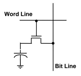
1 Transistor (+ capacitor) memory element Read: Assert Word Line, Sense Bit Line Write: Drive Bit Line, Assert Word Line Need for Refresh Cycles: storage decay in ms Destructive Read-Out Internal circuits read word and write back
