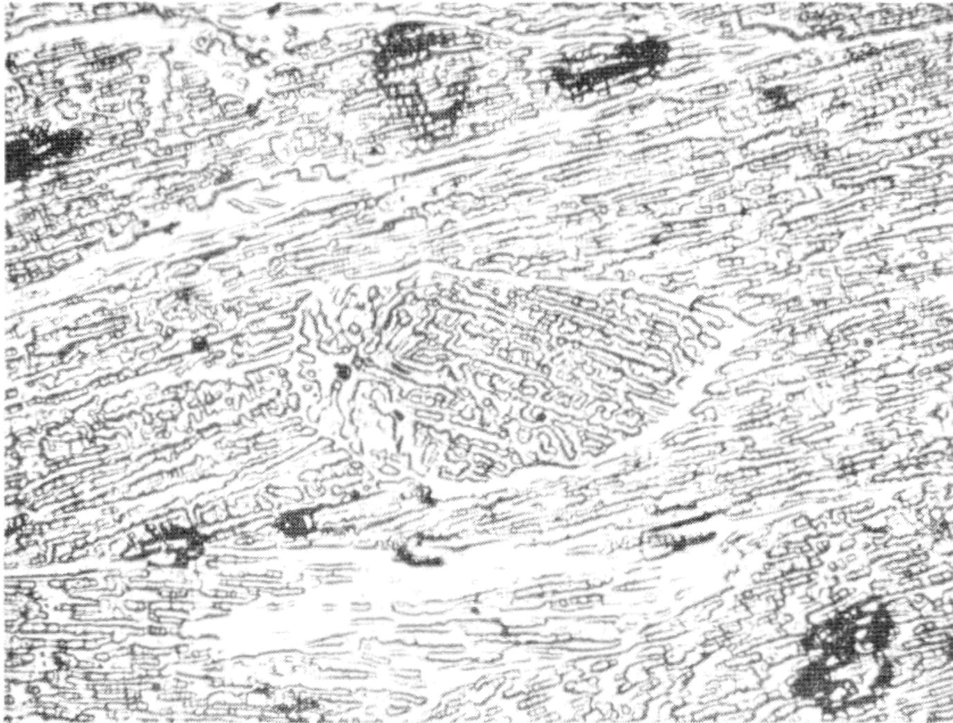
Fig. 8.12. Equiaxed crystals in columnar zone.
