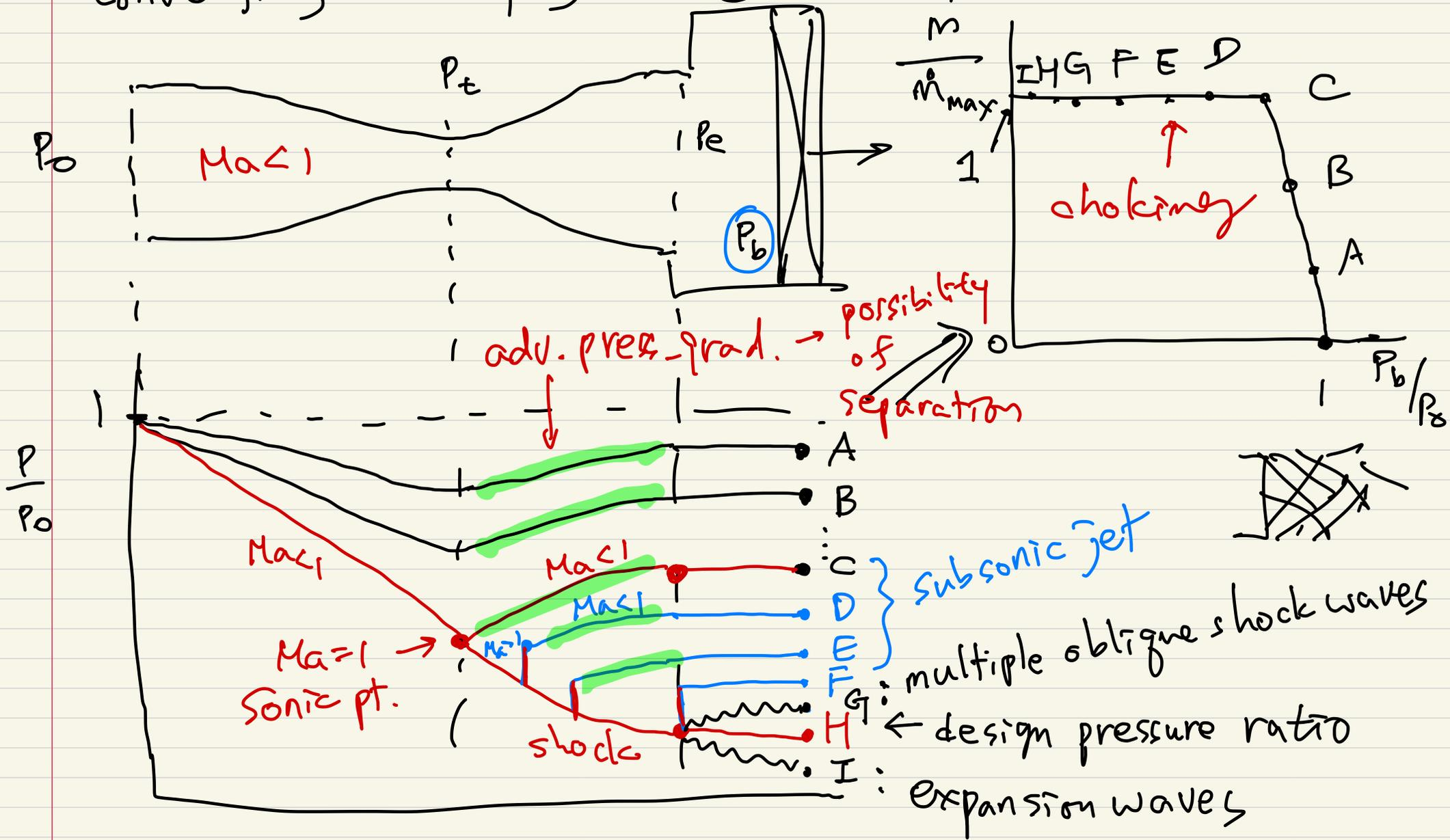
9.7 Compressible duct flow with friction
