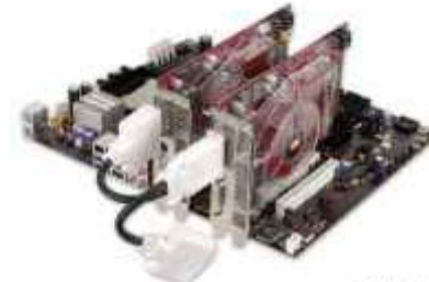
ATI CrossFire Installation
