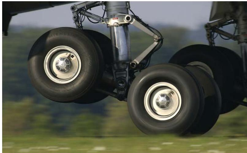
Landing gear system of AIRBUS A330
