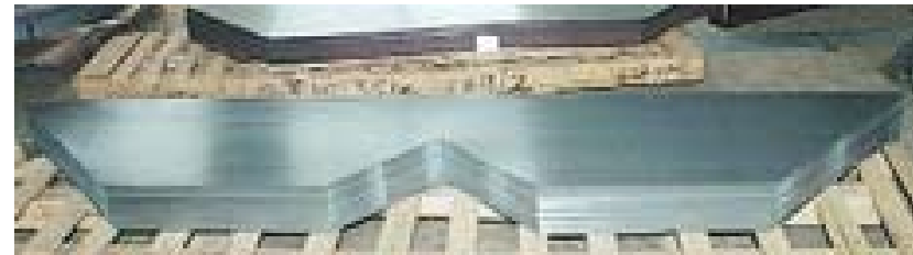
Stacked transformer core
