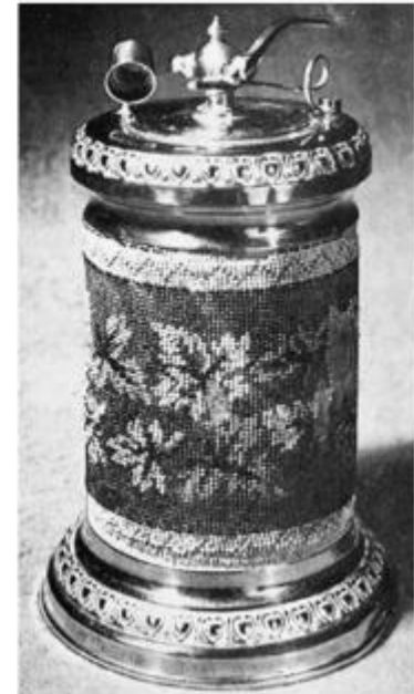
The Döbereiner lighter set-up
