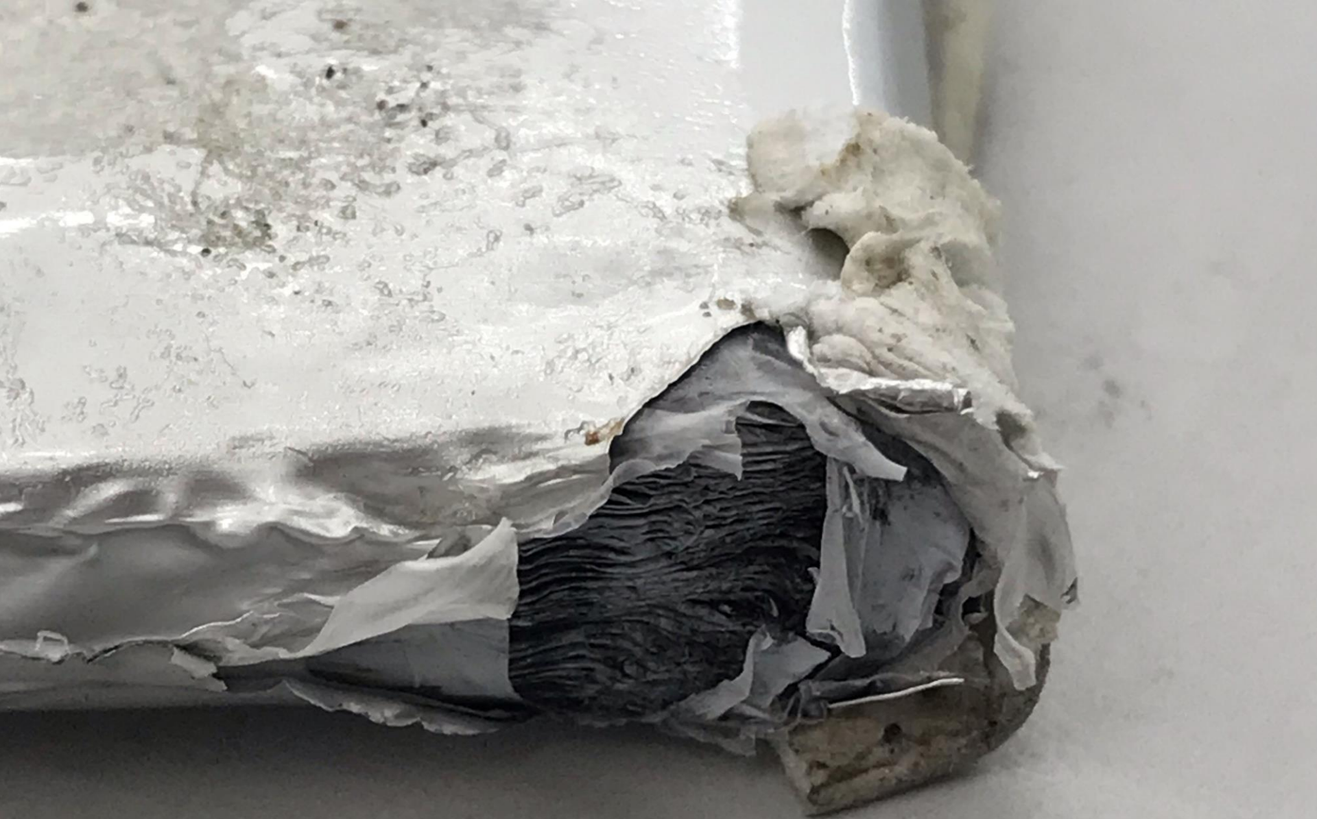
Torn Open and Charred Cell
