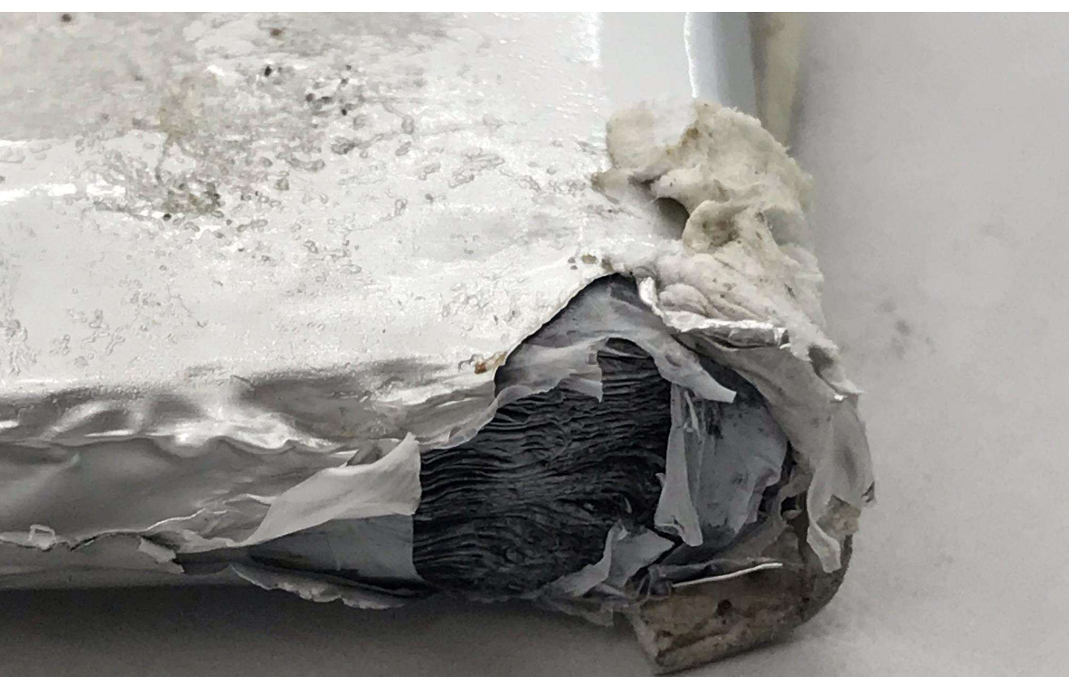
Torn Open and Charred Cell
