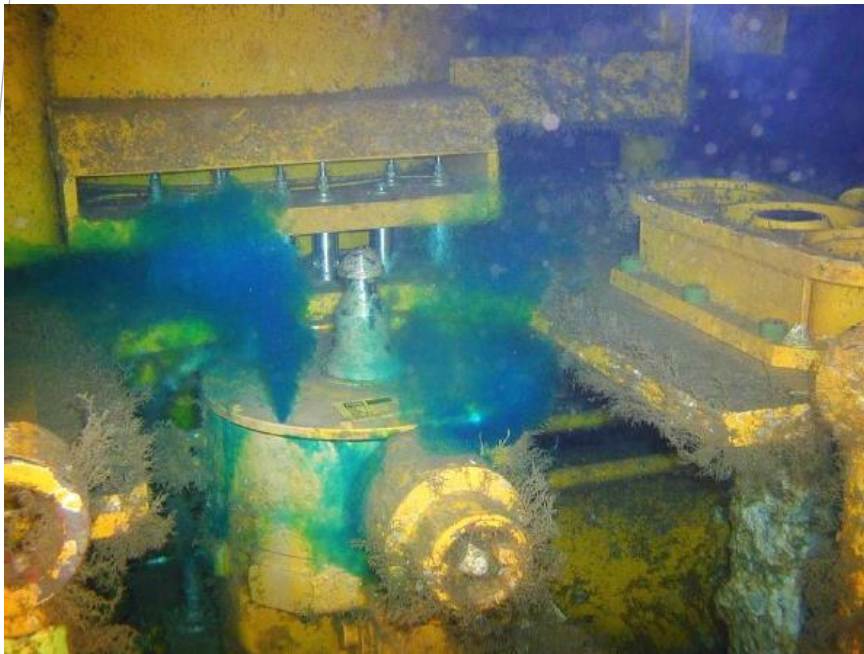
Refraction patterns caused by leaking fluid
