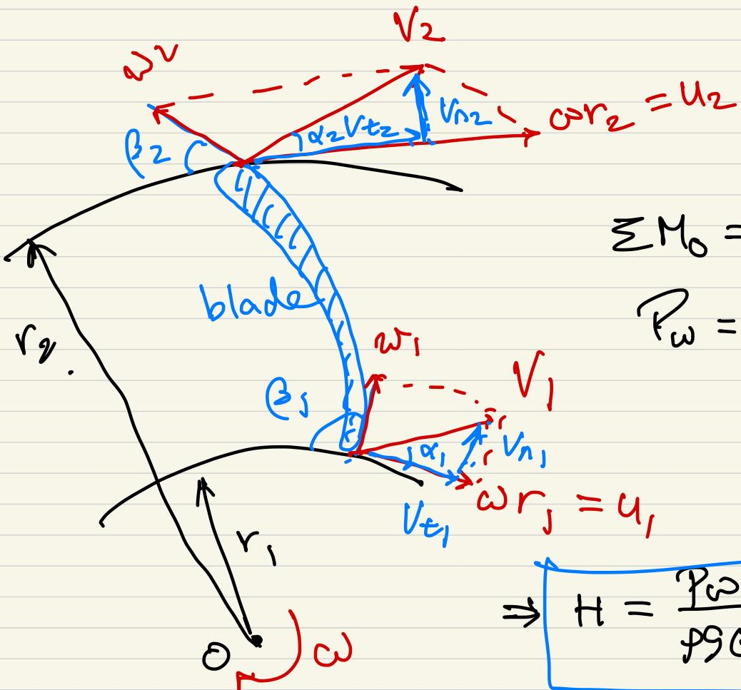
$$\Rightarrow H = \frac{1}{2g} \left[ (V_2^2 - V_1^2) + (U_2^2 - U_1^2) - (W_2^2 - W_1^2) \right]$$
