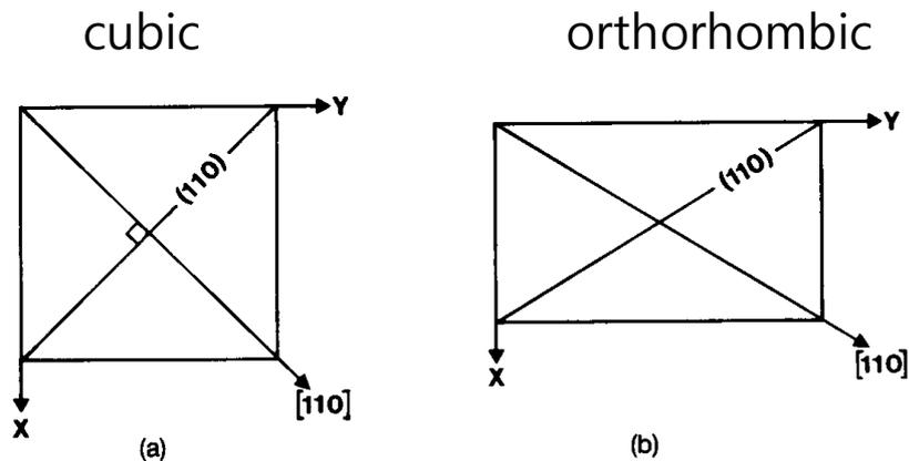
Plans of (a) cubic and (b) orthorhombic unit cells perpendicular to the z-axis, showing the relationships between planes and zone axes of the same numerical indices.
