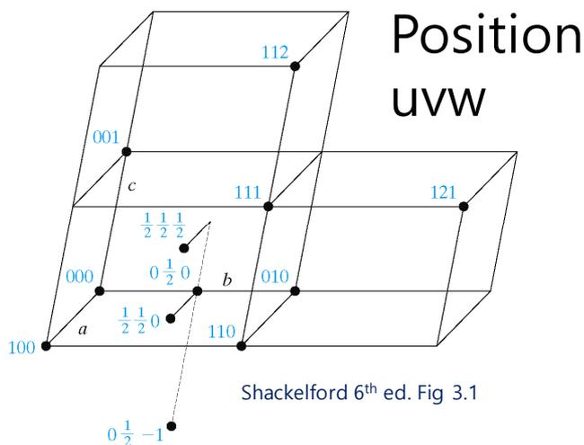
Lattice translations connect structurally equivalent positions (e.g. the body center) in various unit cells
