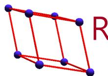
obtained by stretching a cube along one of its axes
