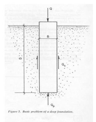
: A cylinder shaft of diameter B is placed to depth D inside a soil mass of known physical properties (c,  $\phi$ ,  $\chi$ ). a static, vertical and central load Q is applied at the top and increased until a shear failure in the soil is produced. <u>the problem is to determine the ultimate load  $Q_0$  that this foundation can support.</u>
