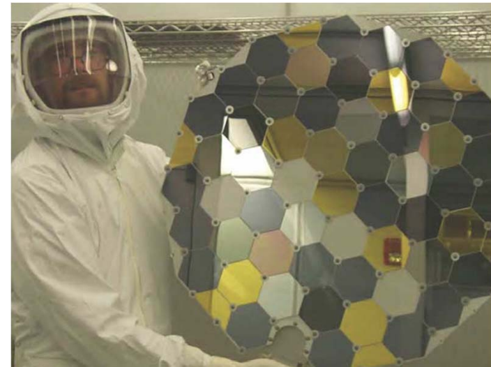
Fig. (a) Artist's impression of the Genesis spacecraft in collection mode, opened up to collect and store samples of solar wind particles. The cover of the canister contains one collector array and the body of a stack of four arrays that can be rotated out when the spacecraft begins its orbit. (b) Genesis' array, held by Andy Stone of the Jet Propulsion Laboratory, showing the collector materials. [(a) courtesy of JPL; (b) courtesy of NASA Johnson Space Center.]
