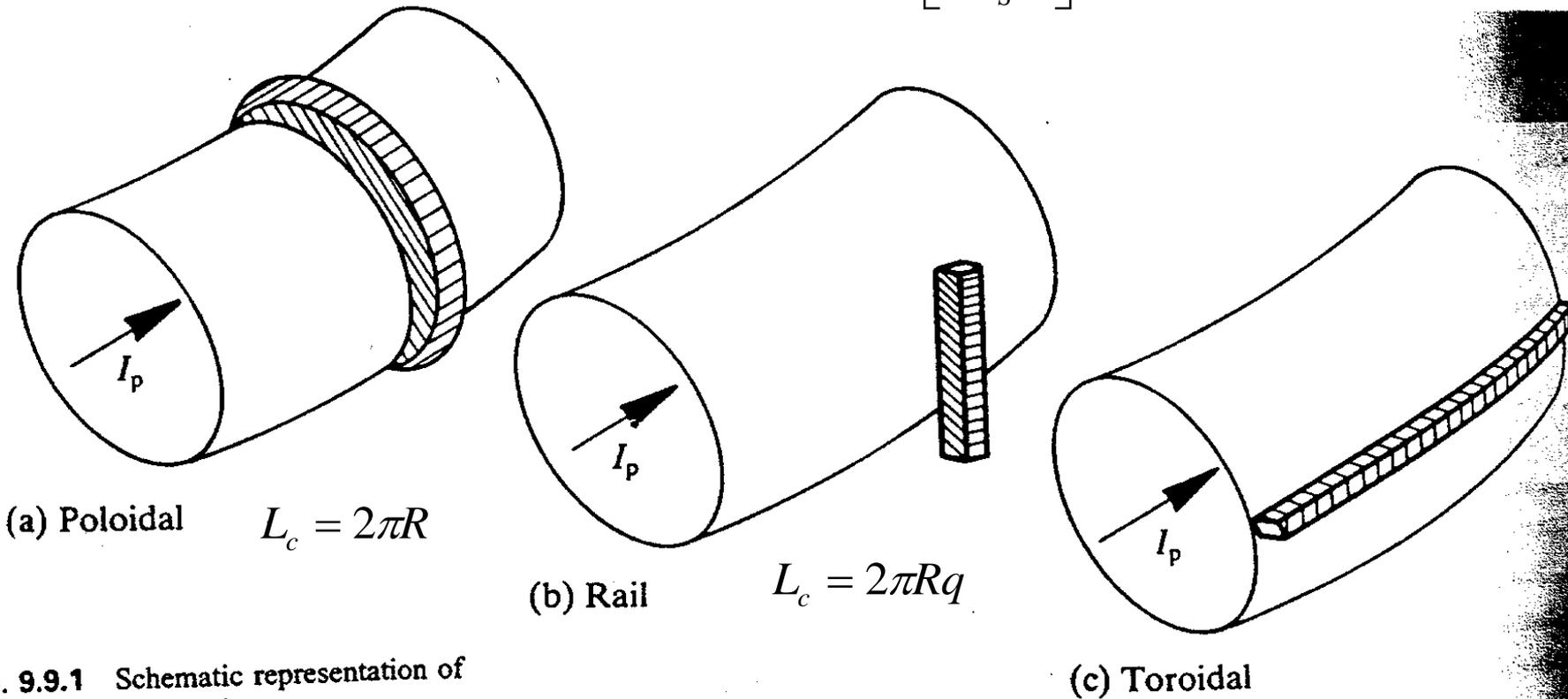
Fig. 9.9.1 Schematic representation of different types of limiter.
