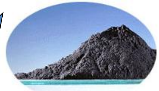
Powdered Activated Carbon (PAC) ; Larger pore diameter than GAC
