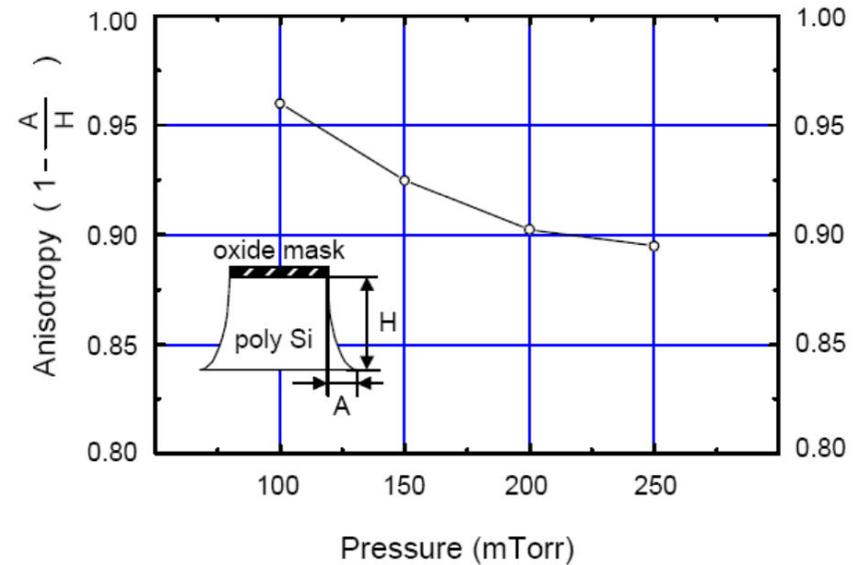
Etch anisotropy as a function of pressure
