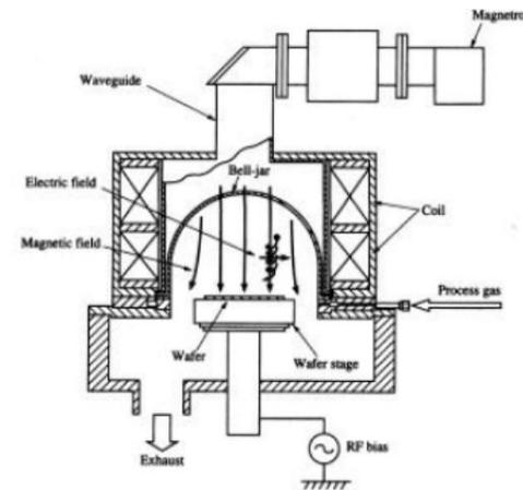
μERIE: microwave electron cyclotron resonance
