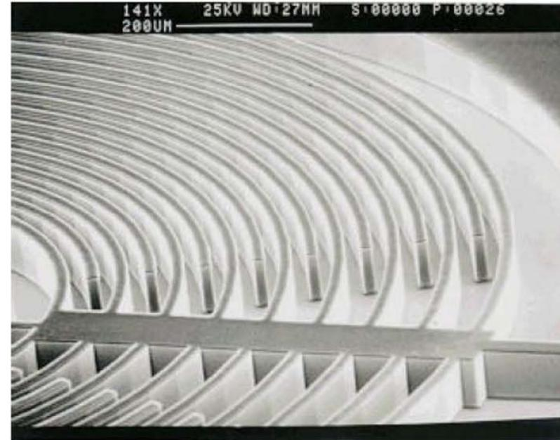
Accelerometer (170 μm-depth)
