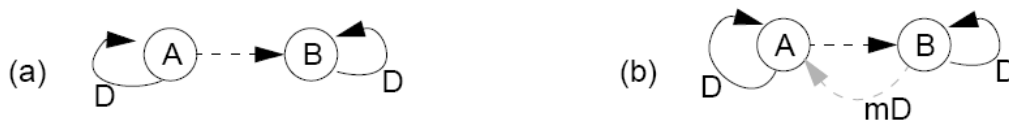
Fig. 2. An IPC graph with a feedforward edge: (a). original graph (b). imposing bounded buffers.
