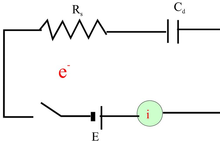
e.g.,)  $R_s = 1 \Omega$ ,  $C_d = 20 \mu\text{F}$ ,  $\tau = 20 \mu\text{sec}$   $\rightarrow$  double layer charging is 95 % complete in  $60 \mu\text{sec}$
