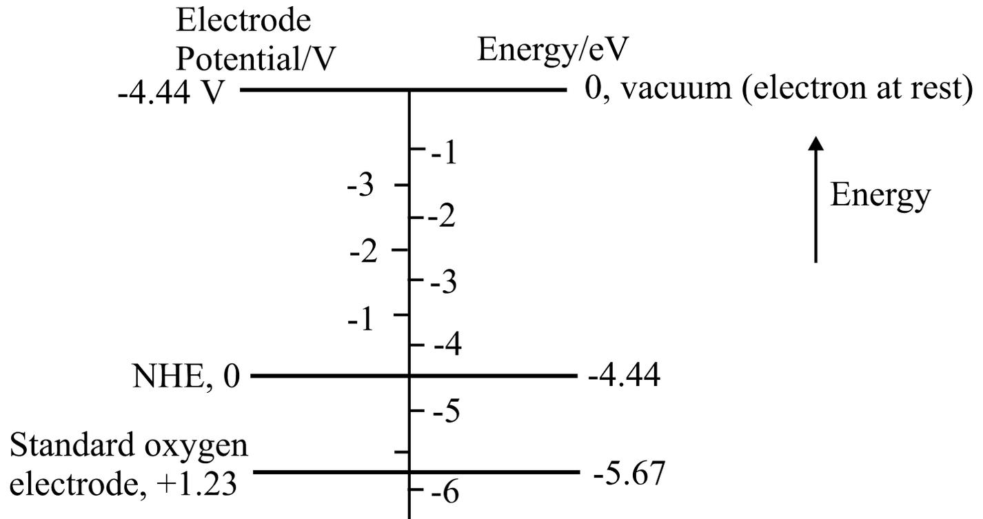
Controlling potential of the working electrode with respect to the reference → controlling the energy of the electrons within the working electrode
