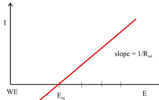
If free of charge transfer and mass transfer overpotentials, slope =  $1/R_{\text{sol}}$
