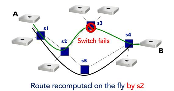
Packet switching beats Circuit switching with respect to resilience and efficiency.
