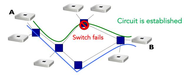
A is forced to signal a new circuit to restore communication.
