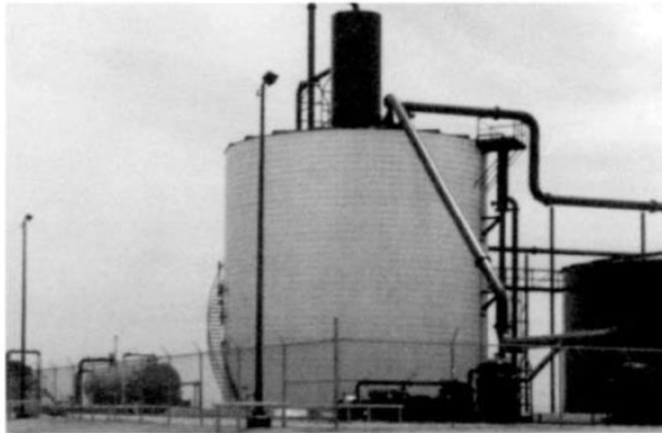
Figure 1-9. A gunbarrel tank for treating oil. The emulsion enters the “gas boot” on top where gas is liberated and then drops into the tank through a specially designed “downcomer” and spreader system. The interface between oil and water is maintained by the external water leg attached to the right side of the tank. Gas from the tank goes through the inclined pipe to a vapor recovery compressor to be salvaged for fuel use.
